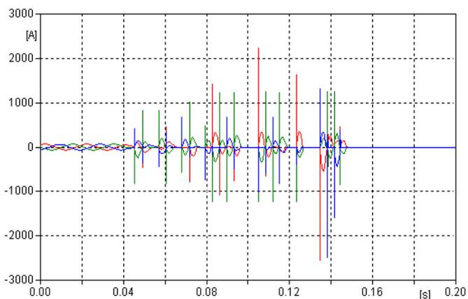
Fig.9. Currents in capacity circuit witch neutral point of battery is insulated and contacts open not simultaneous.
