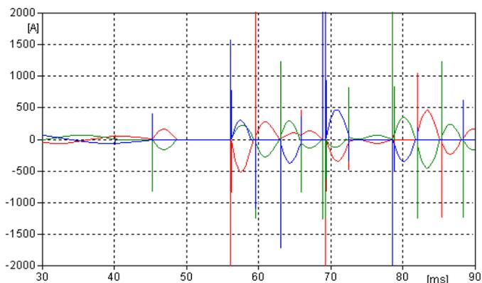
Fig.8 Currents in capacity circuit witch neutral point of battery is insulated and contacts open simultaneous.
