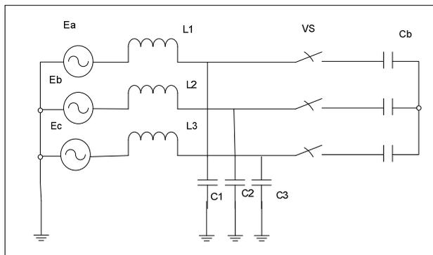
Fig 1 Diagram of simulation model.[2]
