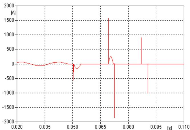
Fig.4 Current on the vacuum switch in capacity circuit witch neutral point of battery is grounded.
