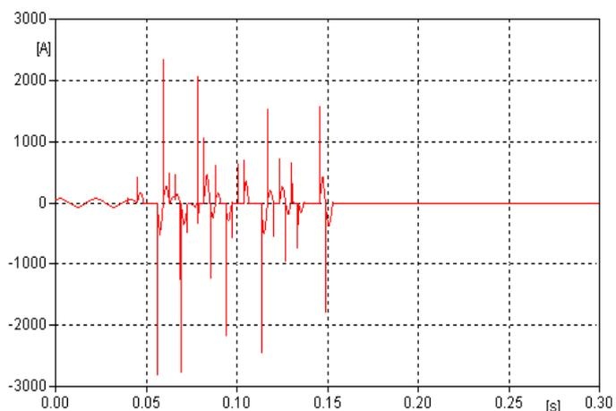
Fig. 5 Current on the vacuum switch in capacity circuit witch neutral point of battery is insulated.
