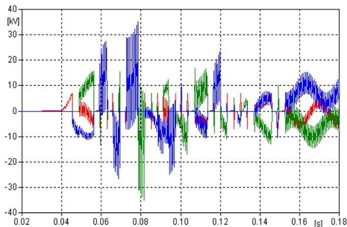
Fig 7 Voltages in capacity circuit witch neutral point of battery is insulated and contacts open simultaneous..
