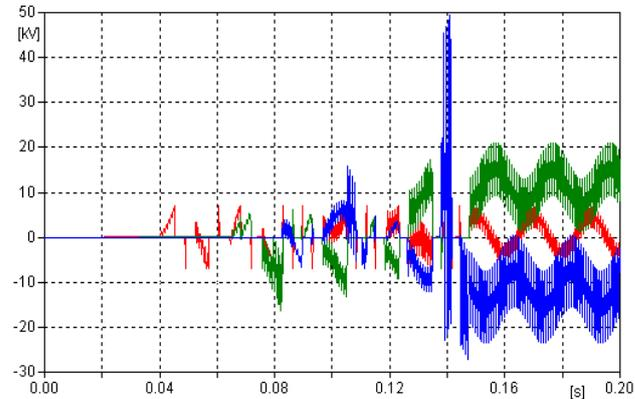
Fig. 6. Voltages in capacity circuit witch neutral point of battery is insulated and contacts open not simultaneous..
