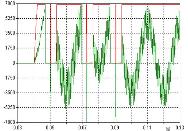
Fig.2 Return voltage (green line) and slop of recovery strength (red line) on the vacuum switch in capacity circuit with neutral point of battery is insulated.
