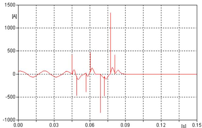
Fig. 11 Current on the vacuum switch in capacity circuit witch neutral point of battery is insulated and two pole open simultaneous.
