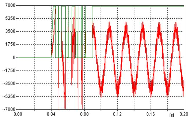
Fig10. Return voltage (green line) and slop of recovery strength (red line) on the vacuum switch in capacity circuit witch neutral point of battery is insulated and two pole open simultaneous.
