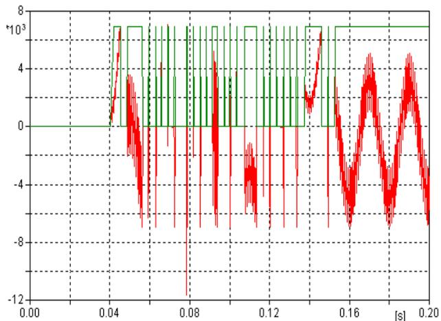
Fig.3 Return voltage (green line) and slop of recovery strength (red line) on the vacuum switch in capacity circuit witch neutral point of battery is insulated.
