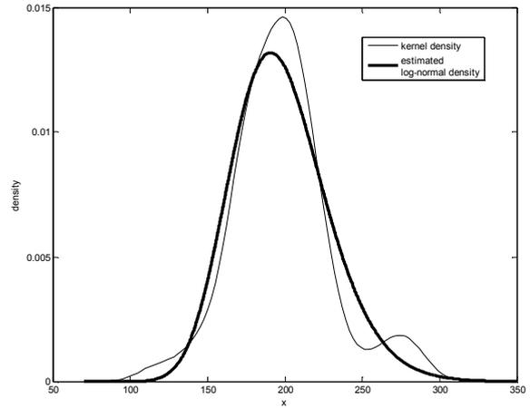
Figure 5. The kernel estimator of density function based on the real power data and the log-normal density with estimated parameters.
