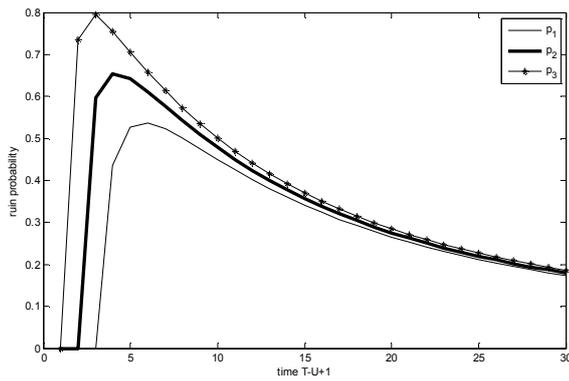
Figure 7. The ruin probability as a function of power delivery time period in stochastic Cournot equilibrium model based on real power data.
