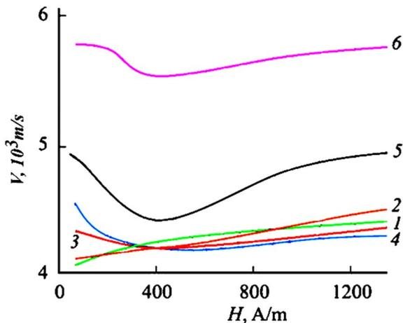
Figure 2. The dependence of propagation velocity of magnetoelastic vibrations on external magnetic field. The annealing of samples is carried out by direct current the density of which is equal to ( $A/m^2$ ): 1 -  $1 \cdot 10^7$ ; 2 -  $3 \cdot 10^7$ ; 3 -  $4 \cdot 10^7$ ; 4 -  $5 \cdot 10^7$ ; 5 -  $6 \cdot 10^7$ ; 6 -  $7 \cdot 10^7$ .
