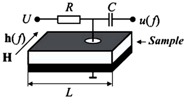
Figure 1. The scheme of experimental investigation of magnetoelastic effect, resonance of magnetoelastic vibrations and obtaining of velocity of their propagation.
