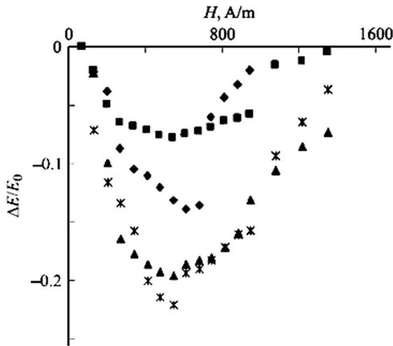
Figure 6. The dependence of  $\Delta E$ -effect value on sample length: 1- 0.06, 2 - 0.05, 3 - 0.04, 4 - 0.03 m
