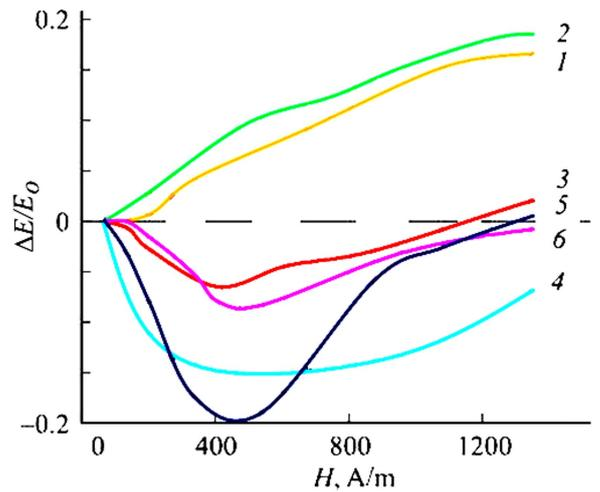
Figure 3. The dependence of relative modulus of elasticity on external magnetic field strength. The annealing of samples is carried out by constant electric field the density of which is equal to ( $A/m^2$ ): 1 -  $1 \cdot 10^7$ ; 2 -  $3 \cdot 10^7$ ; 3 -  $4 \cdot 10^7$ ; 4 -  $5 \cdot 10^7$ ; 5 -  $6 \cdot 10^7$ ; 6 -  $7 \cdot 10^7$ .
