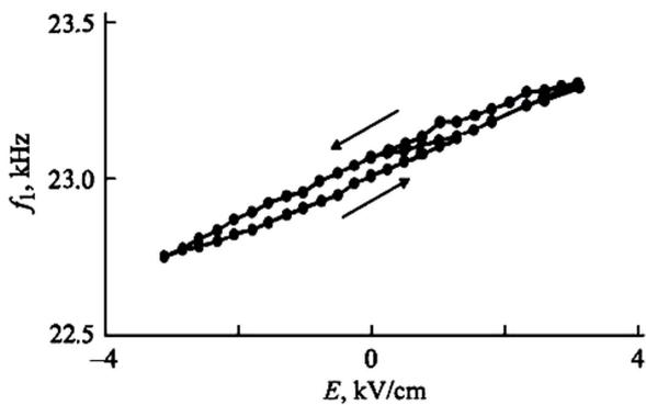
Figure 5. The change of bending vibration frequency in the dependence on electric field strength. It is well seen the hysteresis of bending vibration frequency.
