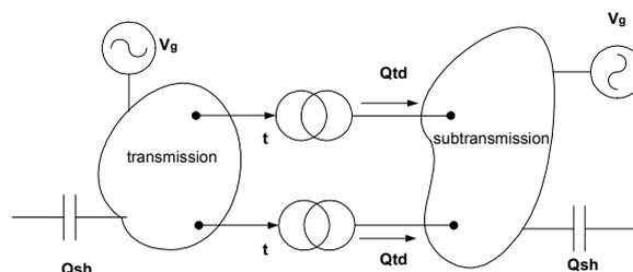
Figure 1. Schematic diagram of a typical T/S power system.
