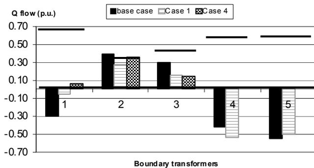
Figure 9. Reactive power flow in boundary transformer.
