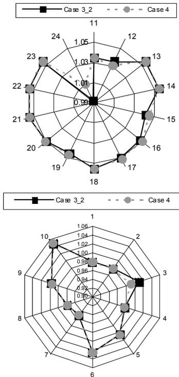
Figure 12. a) Transmission buses voltages; b) Subtransmission buses voltages.
