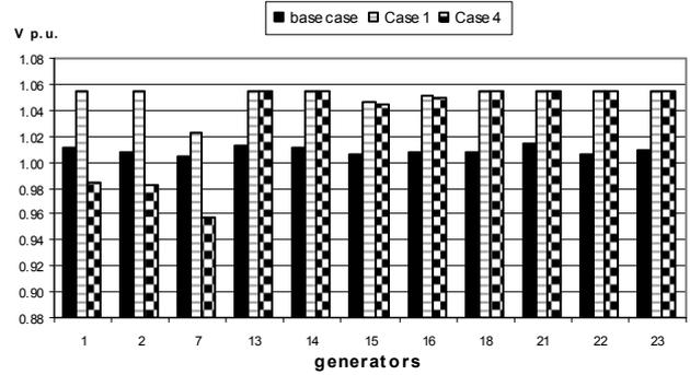
Figure 5. Voltage set-points of generators.
