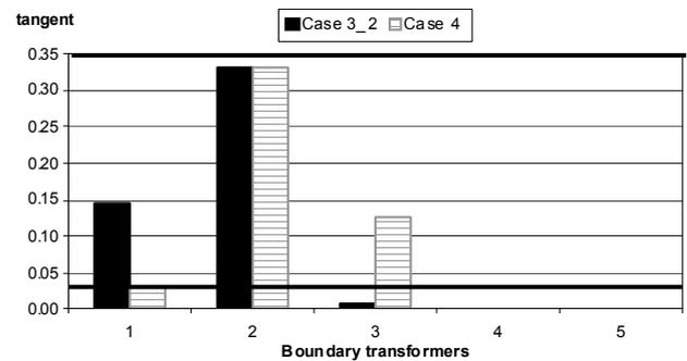
Figure 10. Q/P ratio comparison between case 3\_2 and case 4.
