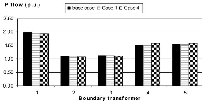
Figure 8. Active power flow in boundary transformer.
