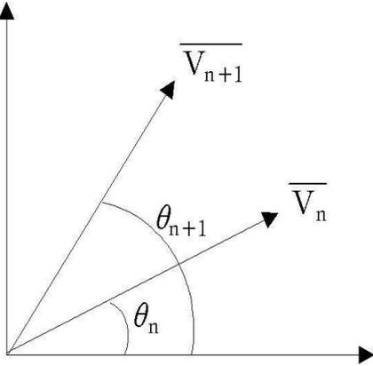
Figure 1. Fundamental frequency phasors corresponding to  $n$  th and  $n+1$  th data windows
