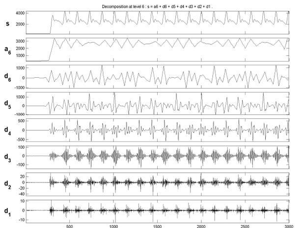
Figure 7. %30 Corrosion faulty motor under %100 load instantaneous power wavelet analysis details
