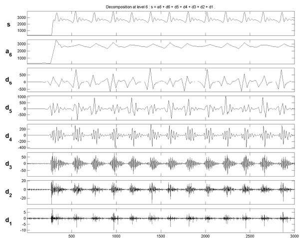
Figure 6. %30 Corrosion faulty motor under %50 load instantaneous power wavelet analysis details
