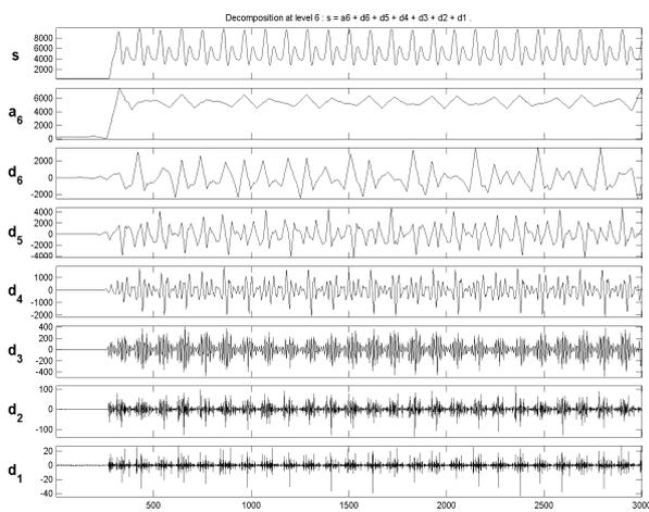
Figure 9. %50 Corrosion faulty motor under %50 load instantaneous power wavelet analysis details
