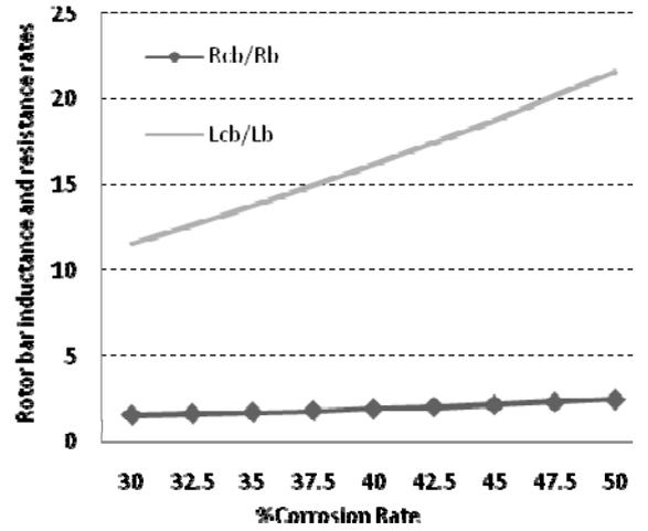
Figure 4. Corrosion rate and rotor bar inductance-resistance rate relation
