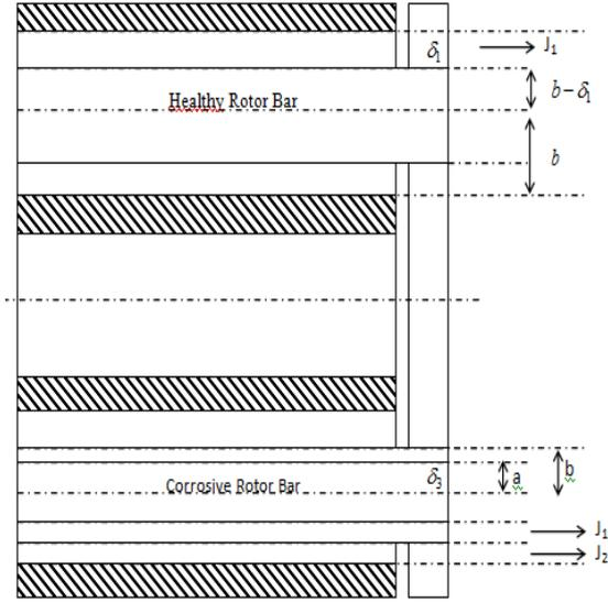
Figure 2. Healthy and corrosive rotor bar model
