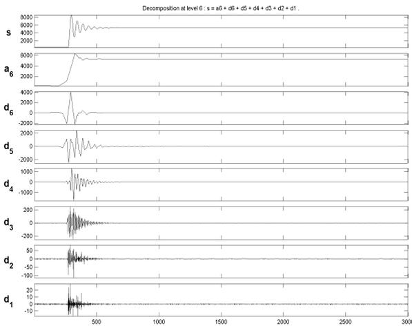
Figure 8. Healty motor under %100 load instantaneous power wavelet analysis details
