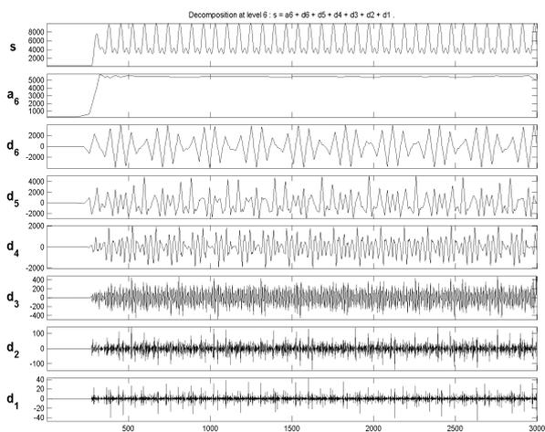
Figure 10. %30 Corrosion faulty motor under %50 load instantaneous power wavelet analysis details
