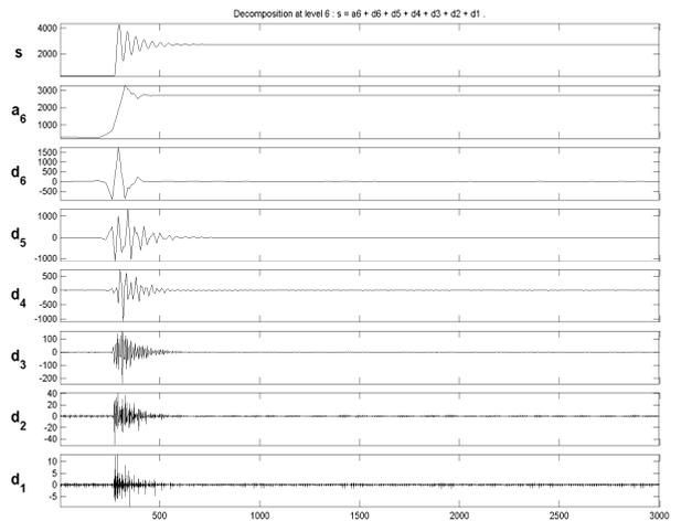
Figure 5. Healthy motor under %50 load instantaneous power wavelet analysis details
