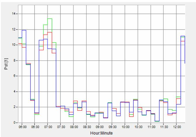
Fig. 7. The  $P_{st}$  flow of the analysed steel plant in the time range from 6:00 to 12:00
