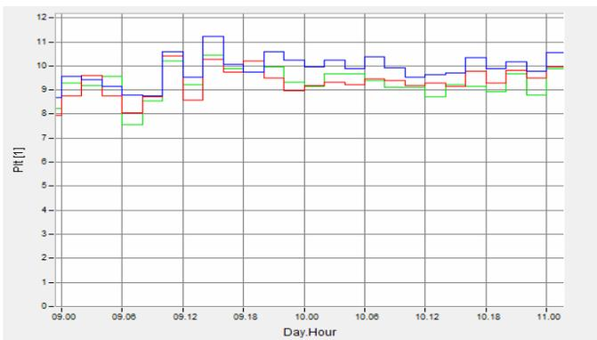
Fig. 8. The 2-day long-term flicker severity  $P_{lt}$  in the steel plant circuits, corresponding to flows from Fig. 5
