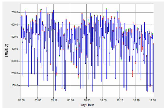
Fig. 5. The exemplary 2-day flows of the voltage (upper picture) and current (lower picture), as 10-minutes averaging RMS values, in the steel plant
