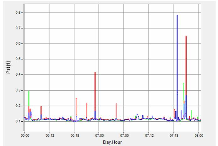
Fig. 2. The 2-day short-term flicker severity  $P_{st}$  in the coalmine circuits, corresponding to flows from Fig. 1
