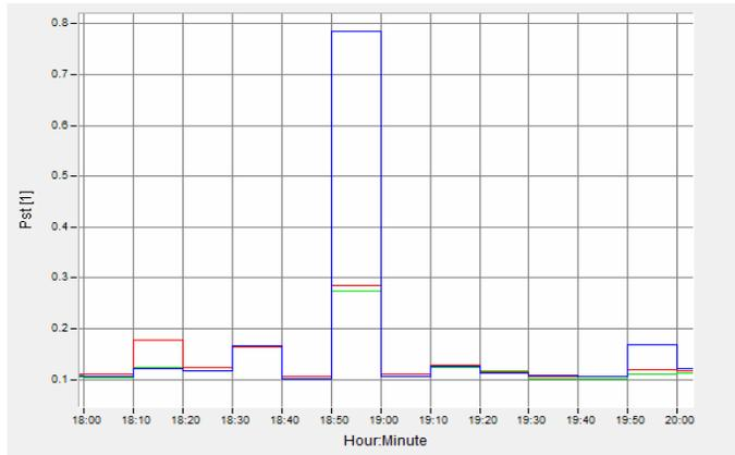
Fig. 3. The  $P_{st}$  flow of the analysed mining machines
