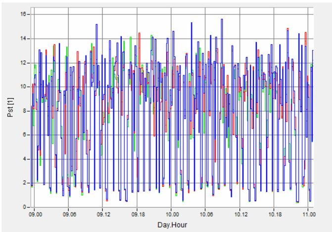
Fig. 6. The 2-day short-term flicker severity  $P_{st}$  in the steel plant circuits, corresponding to flows from Fig. 5
