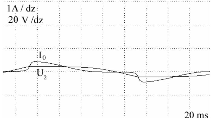
Figure 3. Magnetic current  $I_0$  and secondary voltage  $U_2$  curves in condition of magnetic circuit saturation for magnetic flux strength in the current transformer core equal 40 A/m with no additional conductive disturbances
