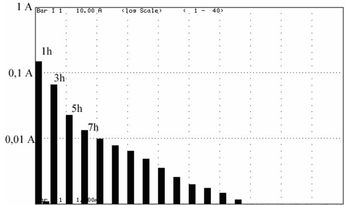
Figure 4. Harmonics of current transformer magnetization current  $I_0$  in condition of magnetic circuit saturation for magnetic flux strength in the current transformer core equal 40 A/m with no additional conductive disturbances
