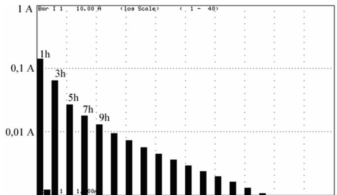
Figure 8. Harmonics of current transformer magnetization current  $I_0$  in condition of magnetic circuit saturation for magnetic flux strength in the current transformer core equal 40 A/m for primary winding supply voltage  $THD_{U_1} = 8\%$
