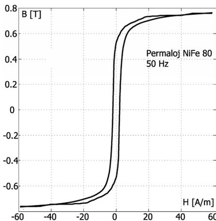
Figure 6. Hysteresis loop of the permalloy NiFe 80 magnetic core determined for primary winding supply voltage frequency 50 Hz with no additional conductive disturbances
