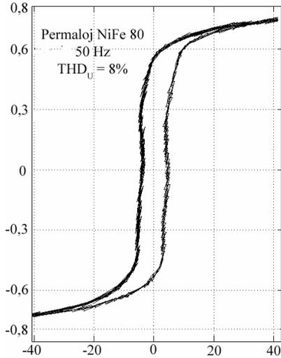
Figure 10. Hysteresis loop of the permalloy NiFe 80 magnetic core determined for primary winding supply voltage frequency 50 Hz and primary winding supply voltage  $\text{THD}_{U1} = 8\%$
