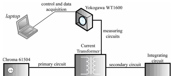
Figure 1. Measuring circuit
