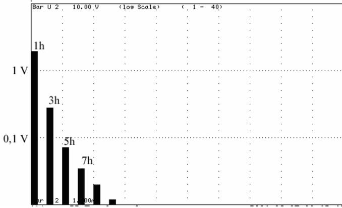
Figure 9. Harmonics of current transformer secondary voltage  $U_2$  in condition of magnetic circuit saturation for magnetic flux strength in the current transformer core equal 40 A/m for primary winding supply voltage  $\text{THD}_{U1} = 8\%$
