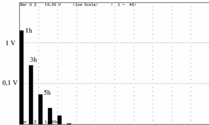
Figure 5. Harmonics of current transformer secondary voltage  $U_2$  in condition of magnetic circuit saturation for magnetic flux strength in the current transformer core equal 40 A/m with no additional conductive disturbances
