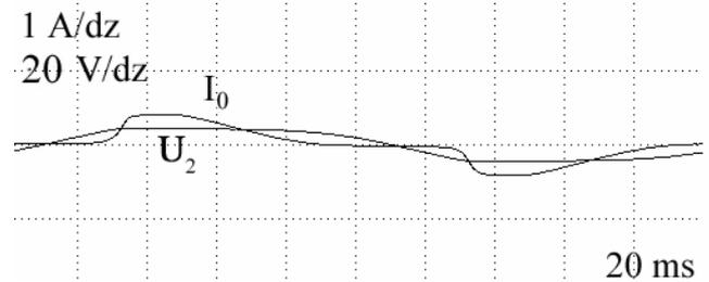
Figure 7. Magnetic current  $I_0$  and secondary voltage  $U_2$  curves in condition of magnetic circuit saturation for magnetic flux strength in the current transformer core equal 40 A/m for primary winding supply voltage  $THD_{U_1} = 8\%$
