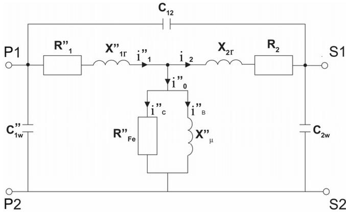
Figure 2. Equivalent circuit of the current transformer with one secondary winding for primary currents frequencies to 10 kHz
