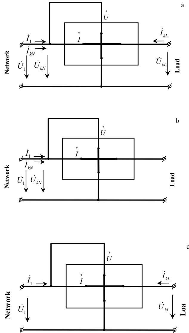
Fig.1. Schemes of meter connection for three cases
