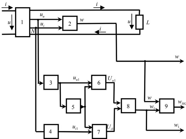
Fig. 3. Generalized schematic diagram of high harmonic energy meter
