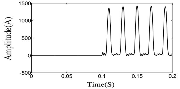
Fig. 6. Typical inrush current.
