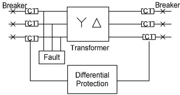
Fig. 5. Three-phase internal fault model.
