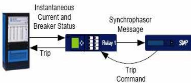
Figure 2. Interconnection of the power system simulator **RTDS**, **relays**, and **SVP**
