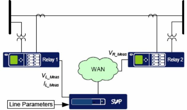
Figure 6. Scheme to supervise remote current and voltage measurements
