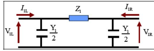
Figure 5. Positive sequence equivalent PI circuit for a transmission line
