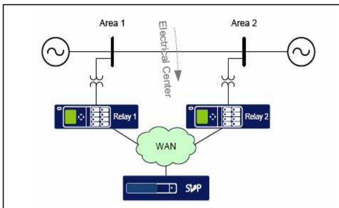
Figure 1. Two-area power systems that uses two **relays** and one **SVP**
