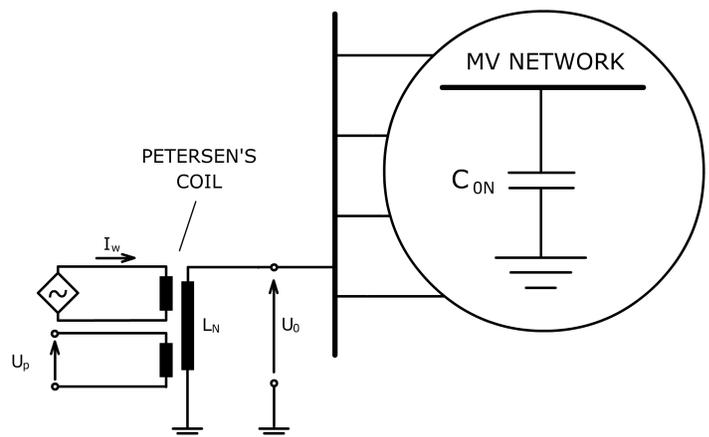
Figure 1. Scheme of equivalent circuit for variable frequency source method.
