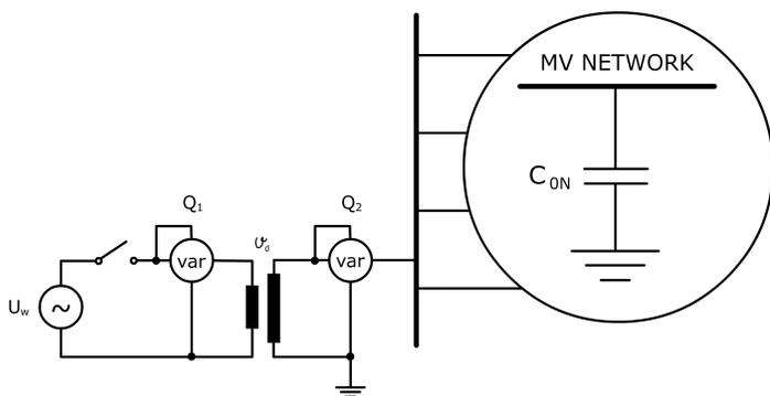
Figure 2. Scheme of equivalent circuit for fixed frequency source method.
