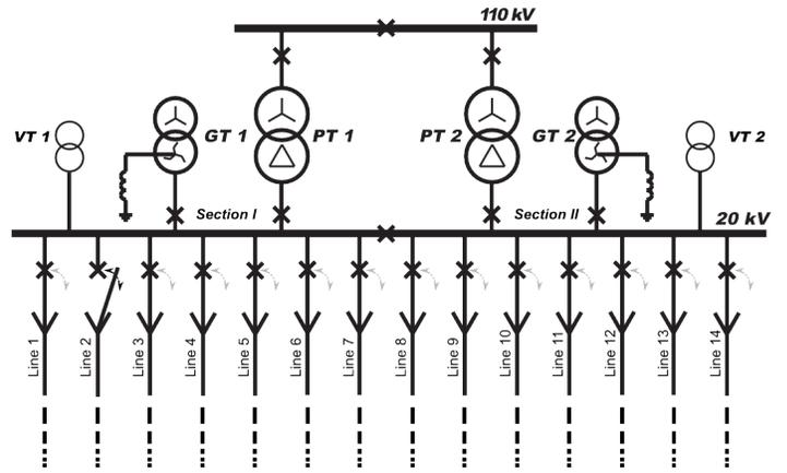
Figure 5. Scheme of 20kV network with disconnected line No. 2.
