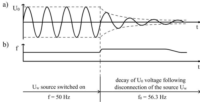
Figure 4. The waveform (a) of the residual voltage and calculated corresponding frequency (b) during measurement process recorded in compensated network ( $s > 1$ ).
