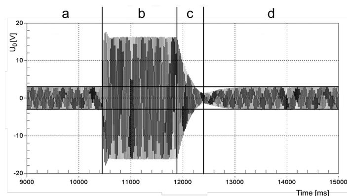
Figure 3. The waveform of the residual voltage recorded during measurements: a) normal operating state, b) additional voltage source connected, c) damped oscillations after additional source disconnection, d) normal operating state.
