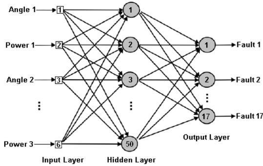
Figure 7. MLP structure used in the Expert System
