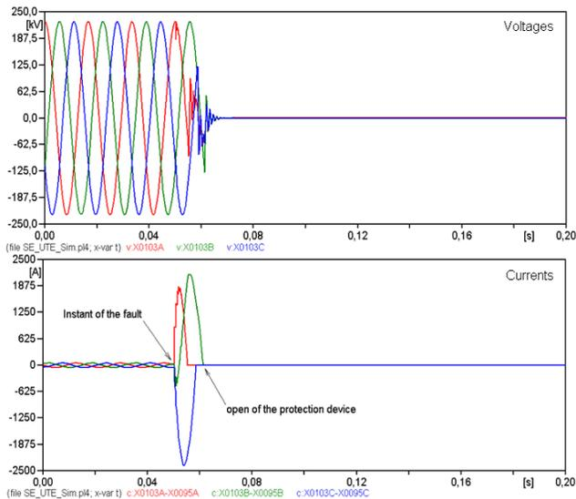
Figure 8. Voltages and currents on Line L1 due three-phase short-circuit.
