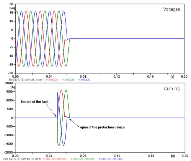
Figure 10. Voltages and currents on out ST generator with fault (no open) of the circuit breaker 52-7.
