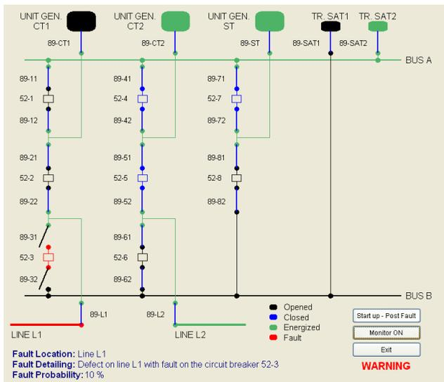
Figure 9. Software interface shows defect in line L1
