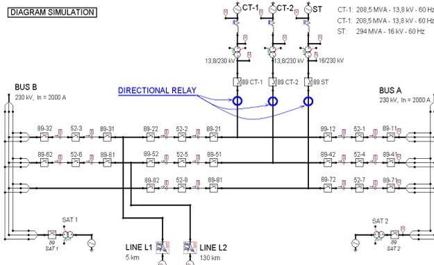
Figure 4. Substation Model.
