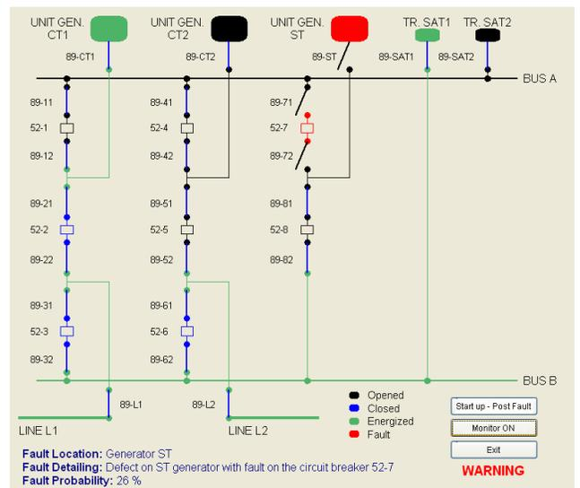
Figure 11. Software interface shows defect in generator ST
