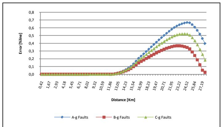
Figure 8. Proposed method for line-to-ground short circuits.
