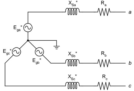
Figure 3. Electrical model of distributed generation to EPDS.
