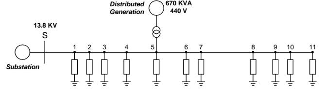
Figure 6. 12 buses system with distributed generation.
