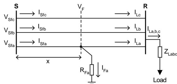
Figure 1. Line-*a*-to-ground fault.
