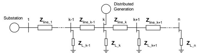
Figure 4. Distribution system with the presence of the DG.
