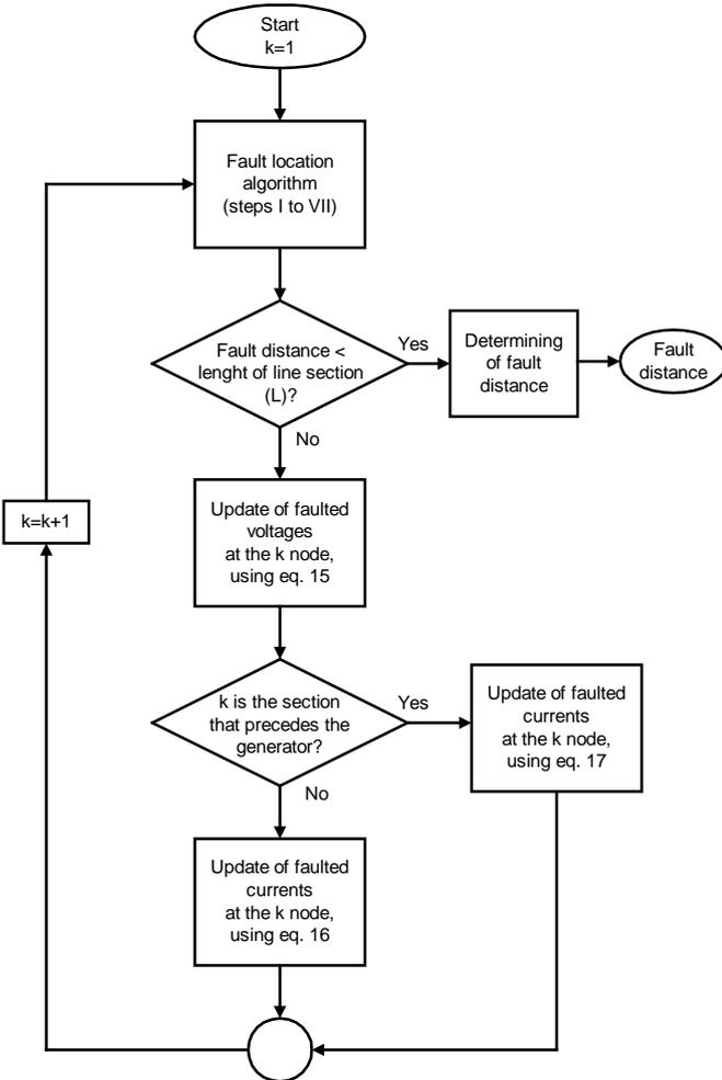
Figure 5. Simplified algorithm to update the voltages and currents.
