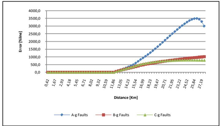
Figure 7. Classical method for line-to-ground short circuits.
