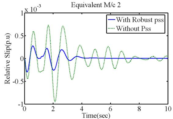
Fig13. Plot of relative slip at equivalent machine 2, with RPSS and CPSS with a 3 phase fault.
