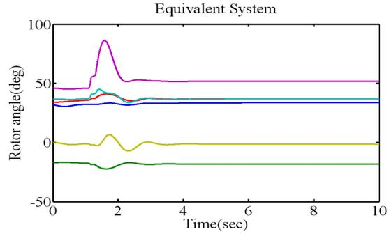
Fig10. Plot of rotor angles at all equivalent machines with RPSS with a 3 phase fault
