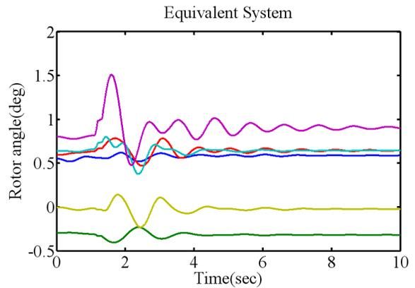
Fig11. Plot of rotor angles at all equivalent machines with CPSS with a 3 phase fault
