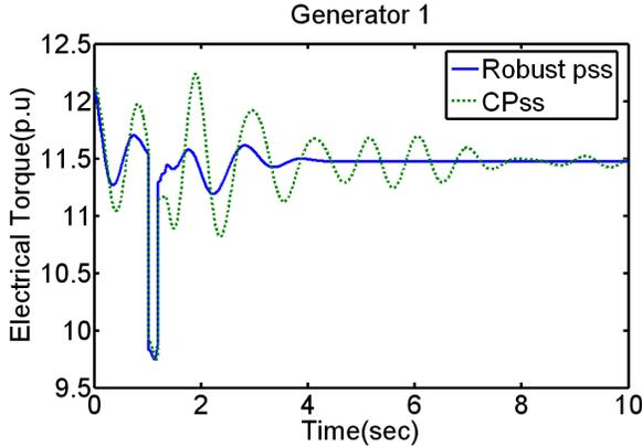
Fig14. Plot electrical torque at equivalent machine 1 with RPSS and CPSS with a 3 phase fault
