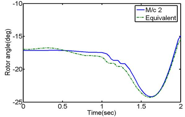
Fig3. Rotor angle plot of M/c 2 and its equivalent.
