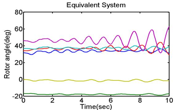
Fig6. Rotor angle at all the machines of equivalent system
