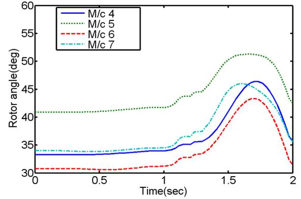
Fig.2. Plot of rotor angle at M/c4, M/c5, M/c6 and M/c7.
