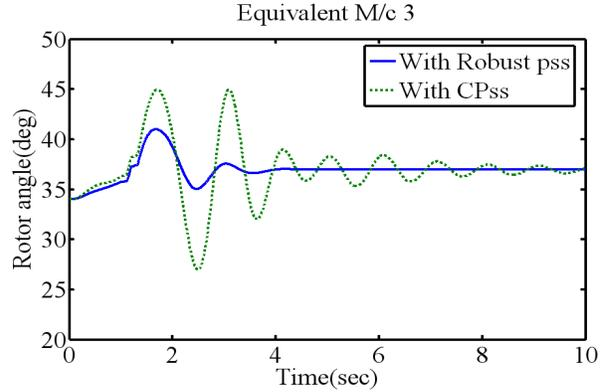
Fig12. Plot of rotor angle at equivalent machine 3, with RPSS and CPSS with a 3 phase fault.
