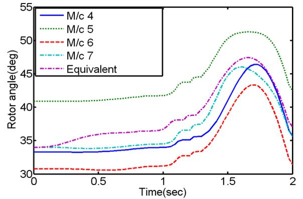
Fig4. Rotor angle plot of M/c 4, M/c 5, M/c 6, M/c 7 and their equivalent
