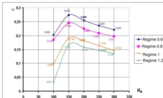
Figure 5. Dependence of damping coefficient on amplification coefficient of AVR+PSS UNITROL-5000 at Shimal TPS at various regimes of power system
