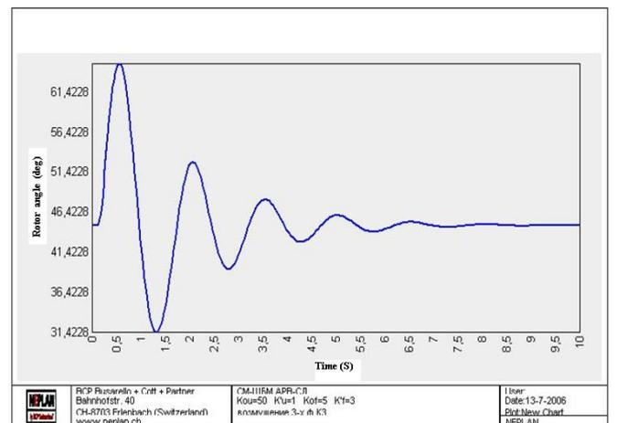
Figure 2. Transient in the Synchronous Machine – Infinite Capacity node scheme, AER-SA:  $K_{ou}=50$ ,  $K'u=1$ ,  $K_f=5$ ,  $K'f=3$
