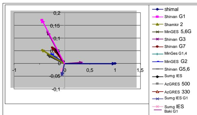
Figure 3. Phasor diagram of distribution coefficients of amplitude of oscillation
