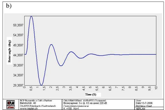
Figure 1. Transient in the Synchronous Machine – Infinite Capability Node scheme AER – UNITROL-5000: a)  $K_A=300$ ,  $K_S=8$ ; b)  $K_A=150$ ,  $K_S=1$
