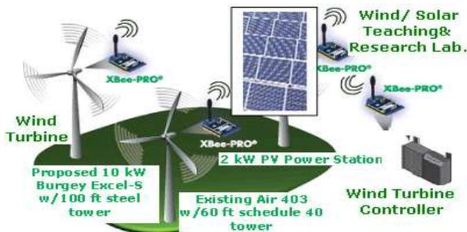
Figure 2. Proposed wireless communication setup among two wind turbines, PV power system located at southwest side of the ITC building, and the main computer located in ITC10 room.
