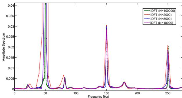
Figure 3. Third simulation, part of the spectrum of the analyzed signal that shows the different accuracy in the recognition of low amplitude components provides by the different value of N for the EDFT algorithm.
