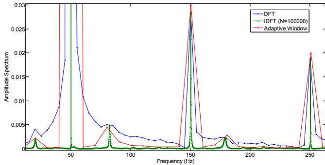
Figure 1. First simulation, part of the spectrum of the analyzed signal that shows the different accuracy in the recognition of low amplitude components provides by the three tested algorithms.
