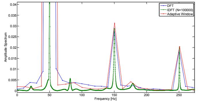
Figure 2. Second simulation, part of the spectrum of the analyzed signal that shows the different accuracy in the recognition of low amplitude components provides by the three tested algorithms.
