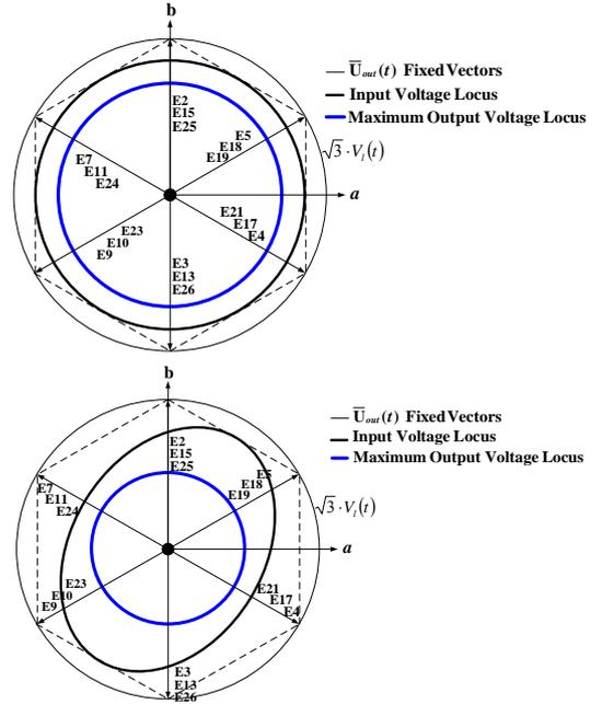
Figure 8. Top: Voltage vectors for balanced input voltage condition. Bottom: Voltage vectors for unbalanced conditions (sag of 50% on phase b)
