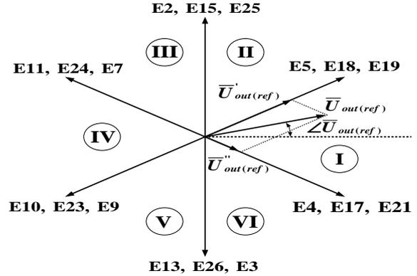
Figure 6. Fix vectors of the output-voltage
