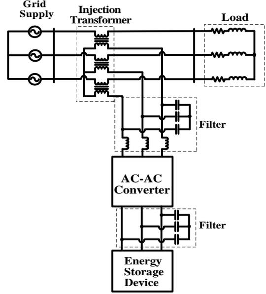
Figure 3. AC/AC DVR without energy storage devices
