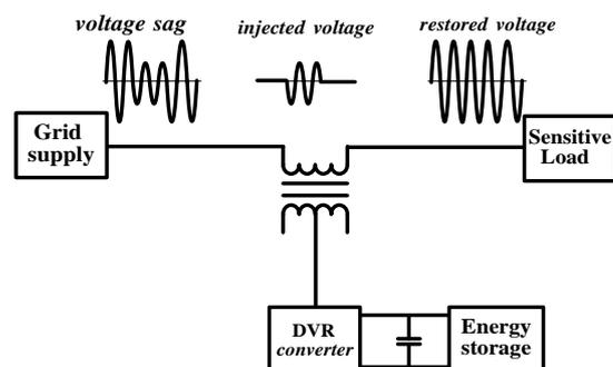
Figure 1. Principle of operation of the dynamic Voltage Restorer
