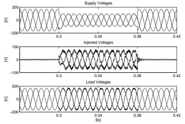
Figure 10. DVR response for balanced voltage sag compensation: Supply voltages, Injected voltages, and Load voltages.
