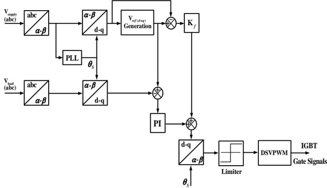
Figure 9. Scheme of the output voltage control based on the PI controller
