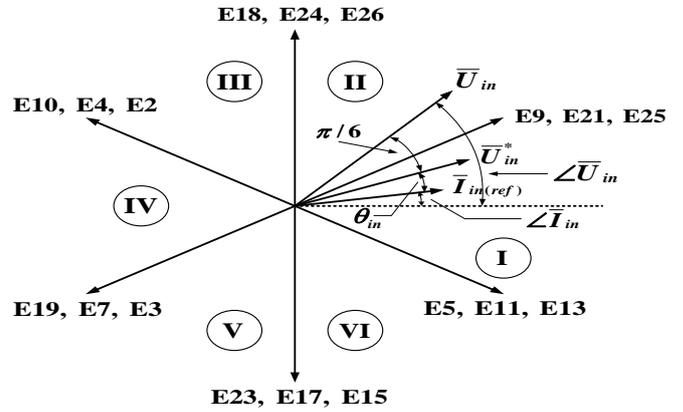
Figure 7. Fix vectors of the input-current
