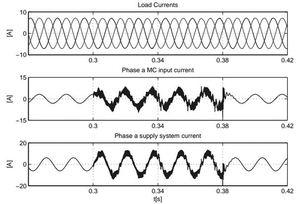
Figure 11. DVR response for balanced voltage sag compensation: Load currents, Phase  $a$  matrix converter input current, Phase  $a$  supply system current.
