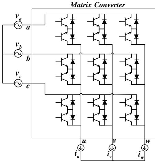
Figure 5. Direct Matrix Converter Topology
