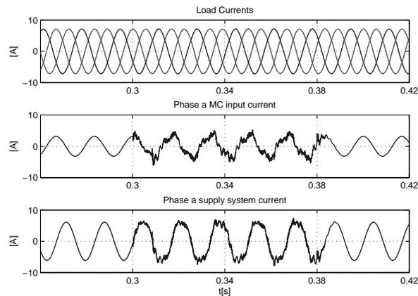
Figure 13. DVR response under unbalanced voltage variation: Load currents, Phase *a* matrix converter input current, Phase *a* supply system current.
