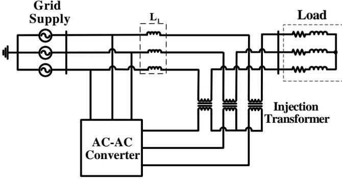
Figure 2. AC/AC DVR without energy storage devices
