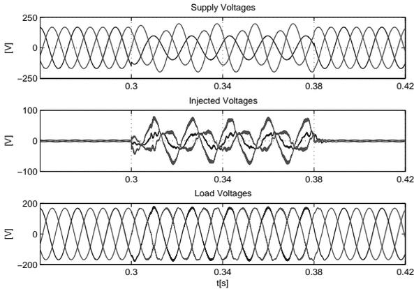
Figure 12. DVR response under unbalanced voltage variation: Supply voltages, Injected voltages, and Load voltages.
