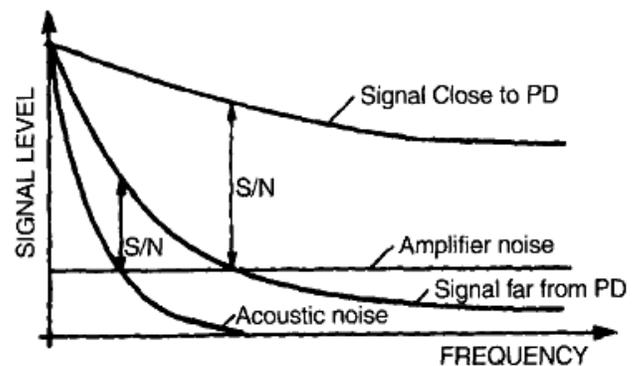
Figure 3: Signal and Noise vs. Frequency, Indicating the Basis for Determining the Acoustic Detection Bandwidth that Provides Optimum Signal to Noise Ratio [1]
