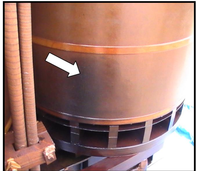
Figure 11 : Burned Insulation
