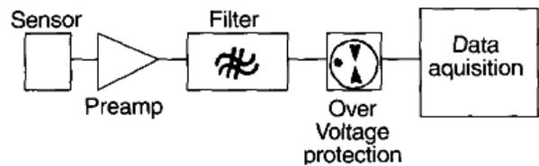
Figure 2: Acoustic PD Detection Circuit [1]
