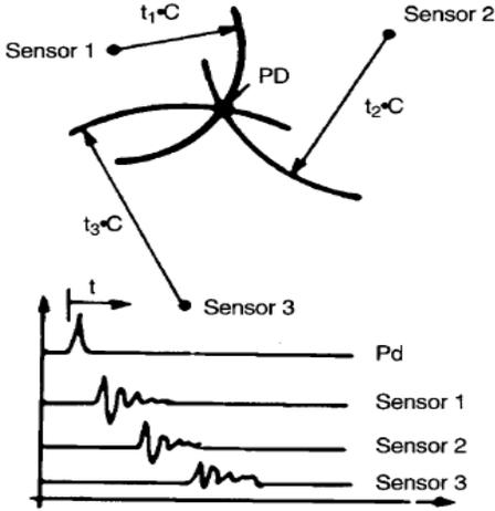
Figure 4 (a): Triangulation of Source Location Based on Time of Flight Measurements Based on Measurement of both Electric and Acoustic Methods [1]
