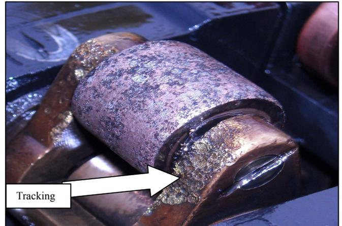
Figure 9: Some tracking observed at the moving contact (T3, T4)
