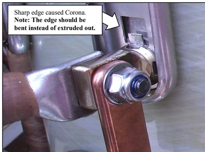
Figure 8: Sharp edges at the OLTC termination (T2, T13, and T14)
