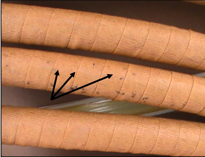
Figure 12: Burned Insulation
