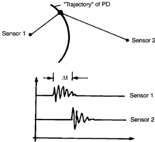
Figure 4 (b): Triangulation of Source Location Based on Time of Flight Measurements Based on Acoustic Methods [1]
