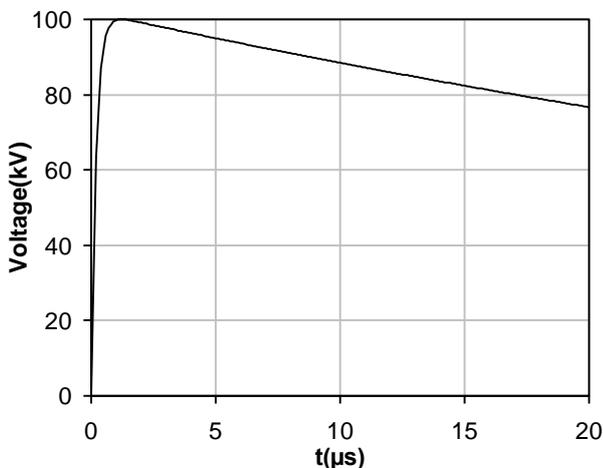
Figure 11. Lightning impulse test voltages for transient simulations.
