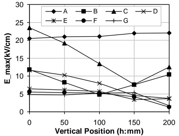
Figure 12. Regional  $E_{\max}$  versus vertical position of the ring. ( $r = 30$  mm,  $D = 200$  mm)
