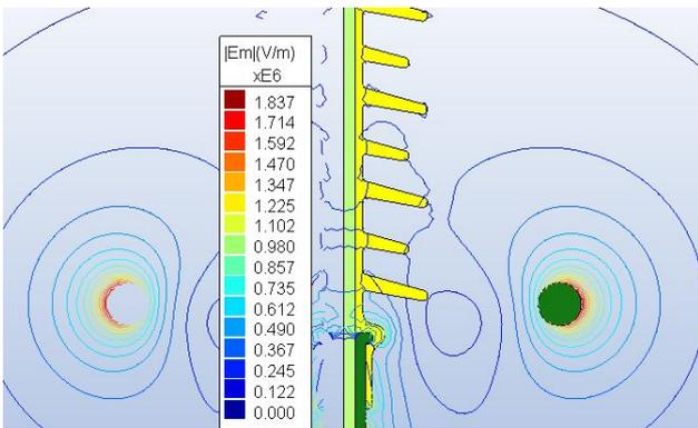
Figure 3. Electrical field contours around silicone insulator
