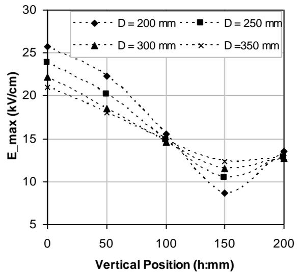
Figure 7.  $E_{max}$  on the critical point C ( $r = 30$  mm)
