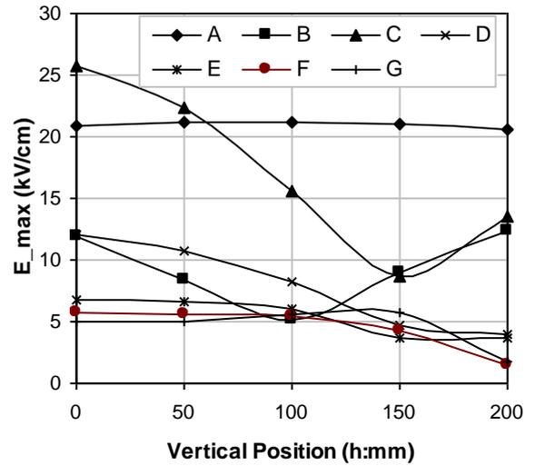
Figure 4.  $E_{max}$  versus vertical position of the corona ring for the critical regions. (r = 30 mm, D = 200 mm)
