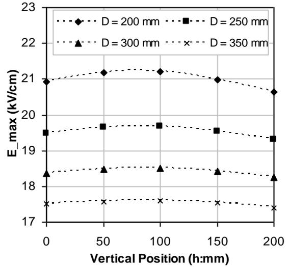
Figure 6.  $E_{max}$  on the corona ring surface, A ( $r = 30$  mm)
