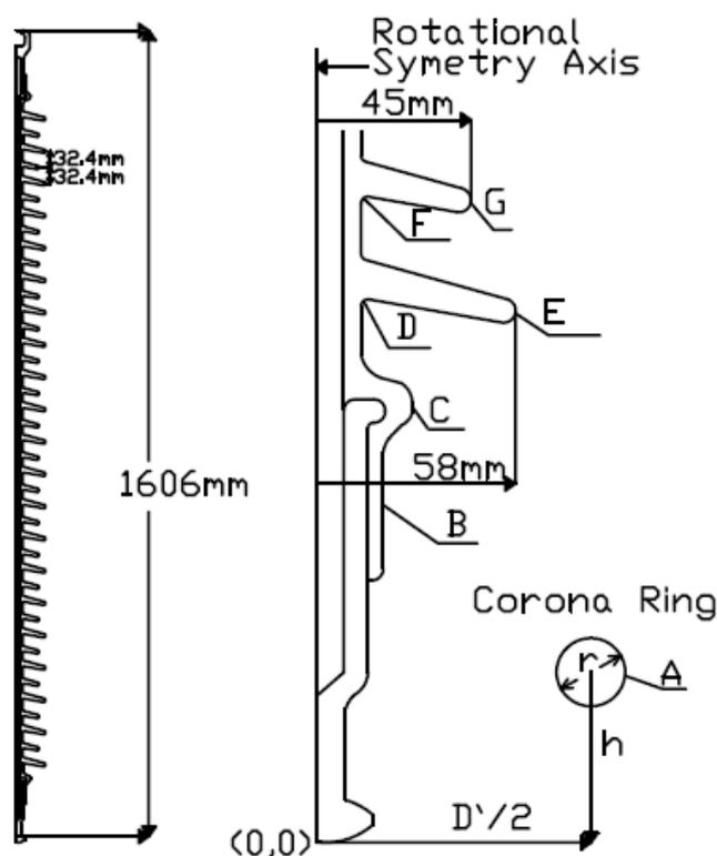
Figure 1. Model of composite insulator and corona ring
