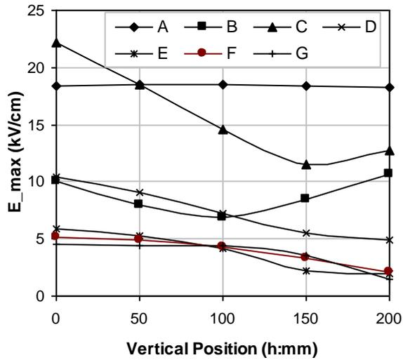
Figure 5.  $E_{max}$  on the critical points ( $r = 30$  mm,  $D = 300$  mm)
