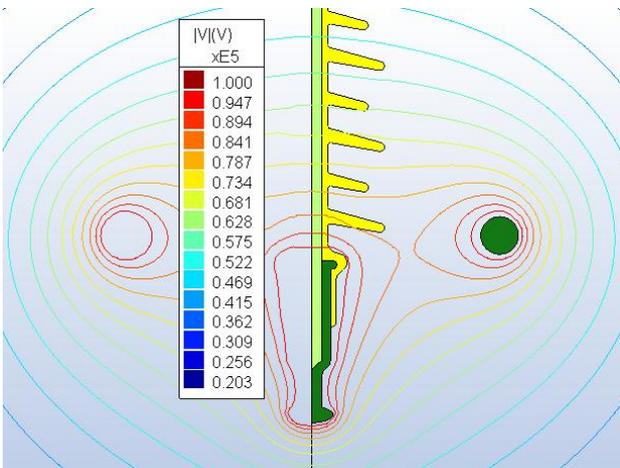
Figure 2. Equipotential contours around silicone insulator
