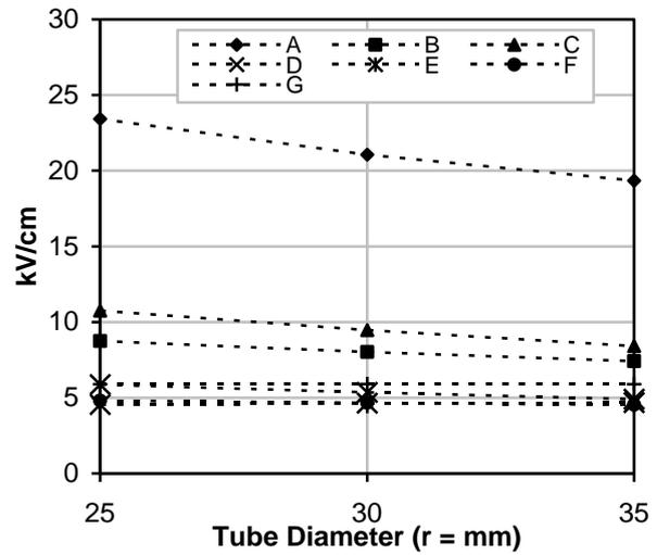
Figure 8.  $E_{max}$  on the critical points (D = 200 mm, h=140 mm)
