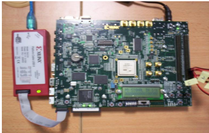
Figure 3 The connection of the FPGA ML405 board Xilinx Virtex 4 and PC are connected by JTAG USB II cables via adaptors for upload the VHDL
