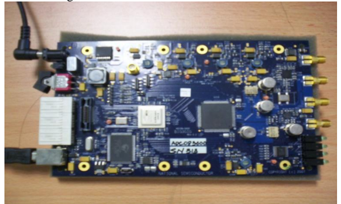
Figure 4 The expansion header to external equipment with 16 LVDS capable differential pairs in ADC083000RB
