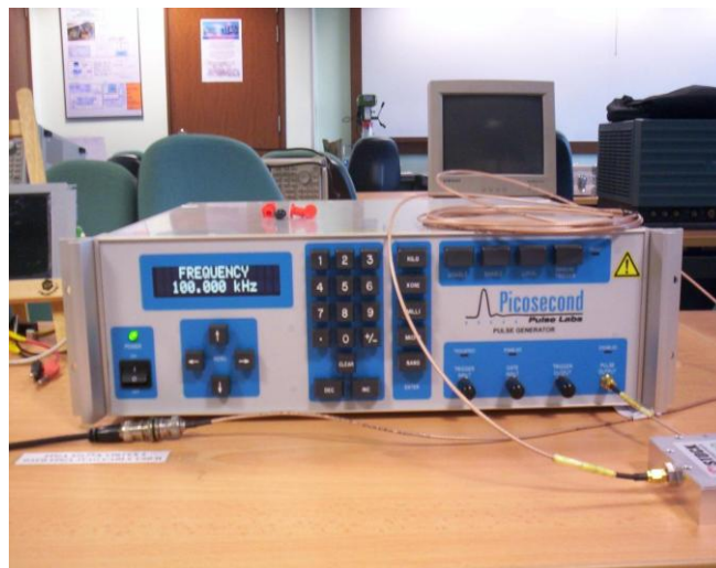
Figure 9 Impulse Generator of PD Detection System
