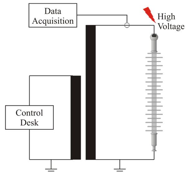
Figure 3. Assembly diagram for measuring leakage current.
