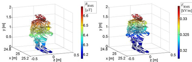
Figure 10. Calculated magnetic and electric fields on the border of overhead line ( $\pm 25$  m) for conductor arrangement obtained by an optimization.
