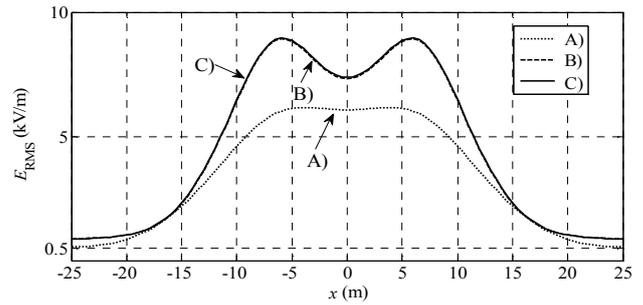
Figure 3. Calculated electric field ( $y = 1\text{m}$ ) of double-circuit overhead power line with two conductor bundle: straight conductor at 2/3 (A) and at 3/3 of sagging (B) and sagged conductor (C).
