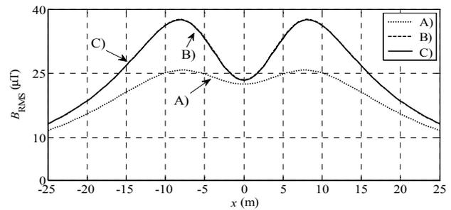
Figure 4. Calculated magnetic field ( $y = 1\text{m}$ ) of double-circuit overhead power line with two conductor bundle: straight conductor at 2/3 (A) and at 3/3 of sagging (B) and sagged conductor (C).
