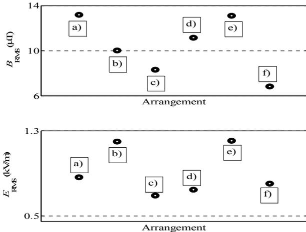
Figure 6. Electric field strength and magnetic field density calculations ( $y = 1m, x = +25m$ ).
