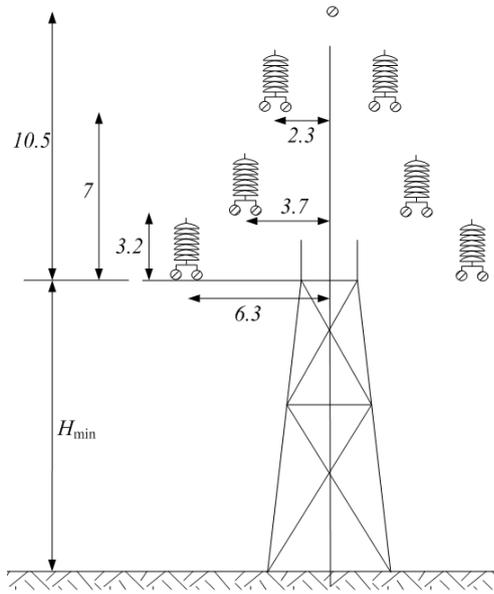
Figure 9. Overhead power line arrangements of two conductor bundle of double tower configuration obtained from optimization process.
