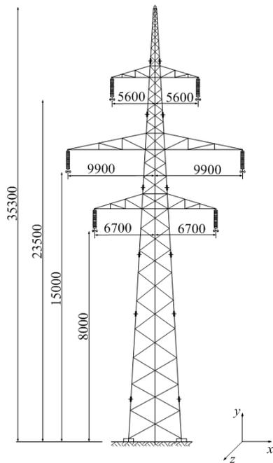
Figure 2. Typical Slovenian double-circuit 400 kV overhead power line.
