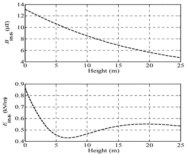
Figure 8. Electric field strength and magnetic field density calculations ( $y = 1m$ ) for the double-circuit Slovenian overhead power lines dependent on the increased height.
