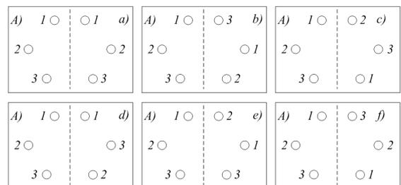
Figure 5. Different conductor sequences of right circuit applied on the double-circuit overhead line.
