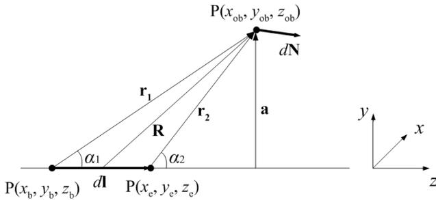
Figure 1. Magnetic and electric field calculation.
