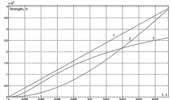
Figure 2. Linear (1), co-sinusoidal (2) and logarithmic (3) laws of circuit-breaker's dielectric strength restoration.
