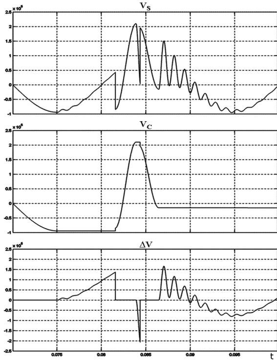
Figure 4. Transitional voltages conditioned by capacitor banks switching-off at use the co-sinusoidal
