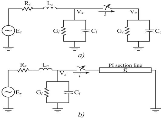
Figure 1. The equivalent networks of connection schemes for the cases of switching-off the capacitor banks (a) and unloaded power transmission line (b). R, L, C and G are resistance, inductance, capacitance and conductance accordingly. Index "s" concerns to the source parameters, "l"- to the load parameters, "c"- to the capacitor banks parameters,  $E_s$  is e.m.f. of voltage source (rms value).
