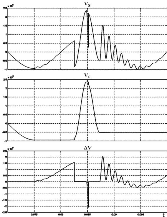
Figure 3. Transitional voltages conditioned by capacitor banks switching-off at use the linear restoration law
