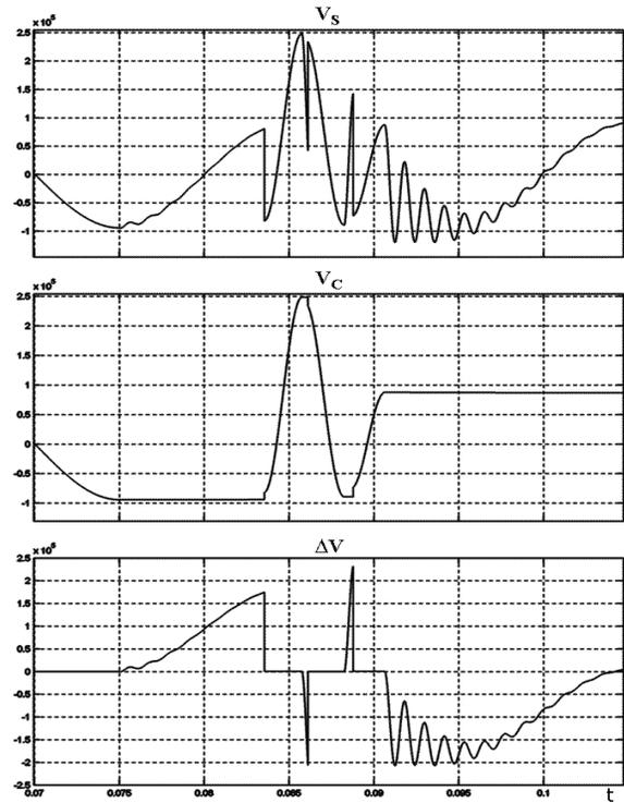
Figure 5. Transitional voltages conditioned by capacitor banks switching-off at use the logarithmic restoration law
