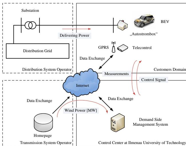
Figure 1. Architecture of the Charging Infrastructure with enhanced Communication Capabilities
