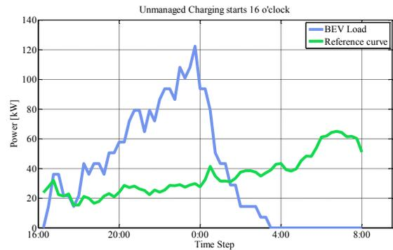
Figure 12. Non optimized Load Shape comparing to the curve to fit
