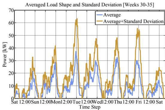
Figure 10. Standard deviation of the five weeks average load shape model
