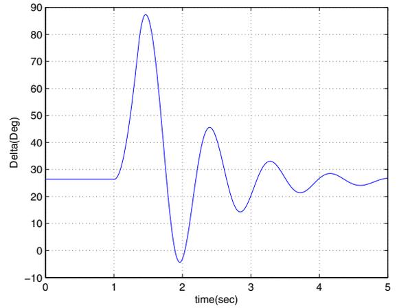
Fig(7): Variation of rotor angle with flatness+RHC based TCSC controller for  $Q=1$  and  $R=1$
