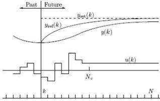
Fig(3):Principle of model predictive control
