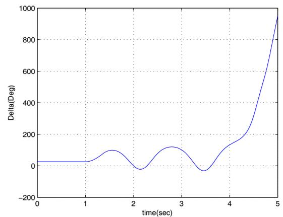
Fig(4):Variation of rotor angle with time without controller
