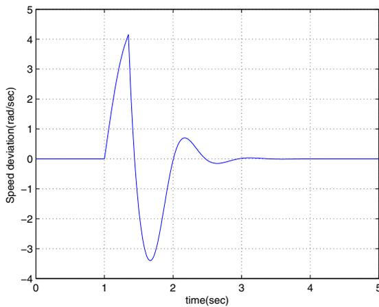
Fig(6): Plot of speed deviation with time using flatness+RHC based TCSC controller for  $Q=0.1$  and  $R=1$
