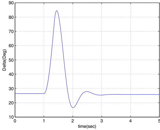
Fig(5): Variation of rotor angle with flatness+RHC based TCSC controller for  $Q=0.1$  and  $R=1$
