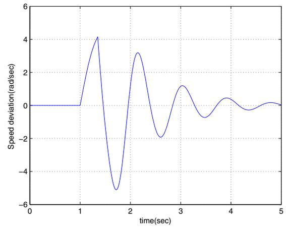
Fig(8): Plot of speed deviation with time using flatness+RHC based TCSC controller for  $Q=1$  and  $R=1$
