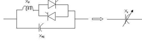
Fig(2): Simplified TCSC model as variable reactance.
