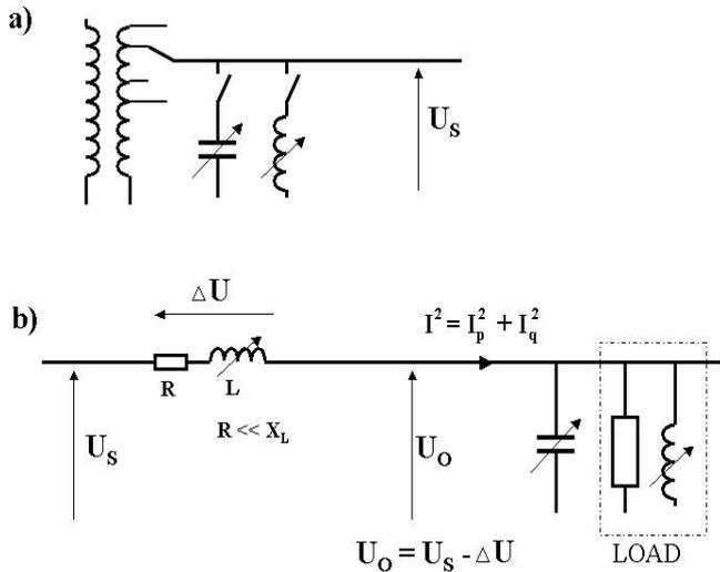
Figure 1. Idea of reactive power and voltage control in the networks.
