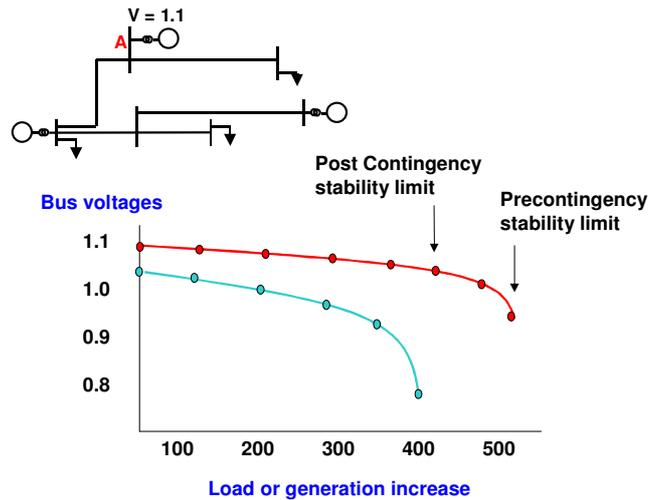
Figure 5. Voltage stability limit is reached when powerflow solution fails to converge
