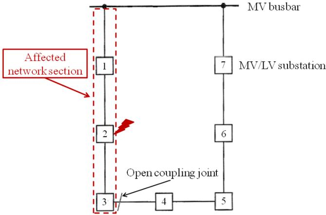
Fig. 3: Affected network section by failure in MV/LV substation 2.
