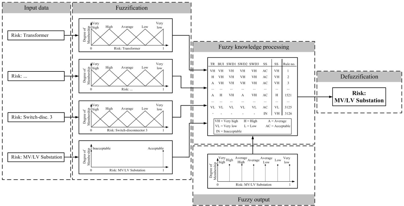
Fig. 5: Configuration of the fuzzy logic system to determine the reversible and irreversible risk carried by a MV/LV substation.
