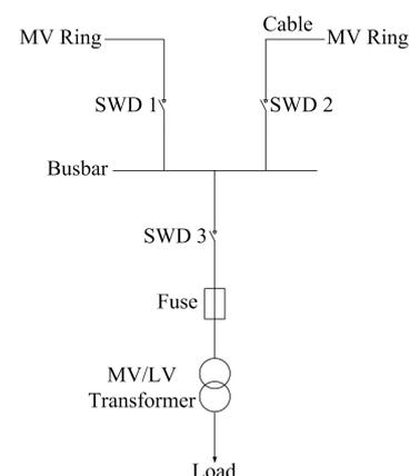
Fig. 1. Block diagram of a MV/LV substation [6].
