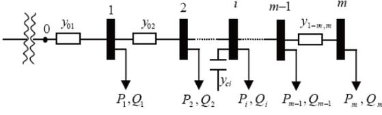
Figure 1. One-line diagram of radial network feeder
