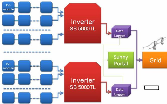
Figure 5. Functional scheme of grid connected PV system
