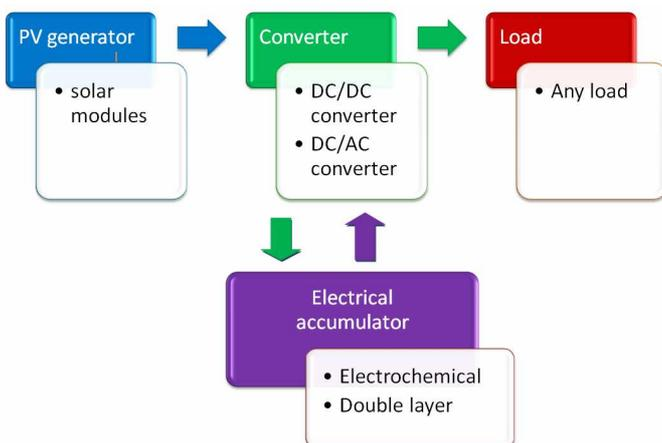
Figure 2. Functional PV-system scheme with energy accumulation.
