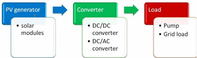
Figure 1. Functional PV-system scheme without energy accumulation.
