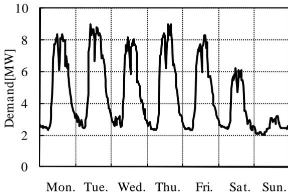
Fig.5 The load curve in demand side for a week
