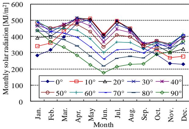
Fig.1 Monthly characteristics of solar radiation depending on the tilt angle in the South
