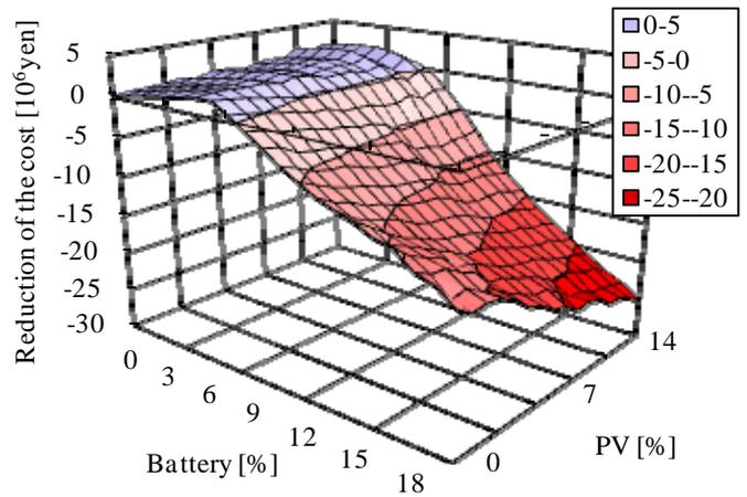
Fig.10 Reduction of total cost depending on BESS and PV
