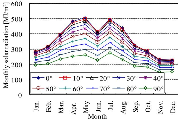
Fig.2 Monthly characteristics of solar radiation depending on the tilt angle in the East and West
