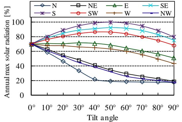
Fig.3 The maximum solar radiation in a year [W/W]
