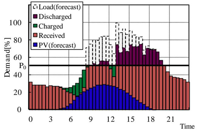
Fig.7 Calculating the target ( $P_0$ ) of receiving power
