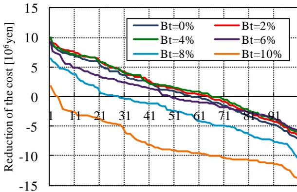
Fig.8 Reduction of total cost by installing BESS (PV=14%)
