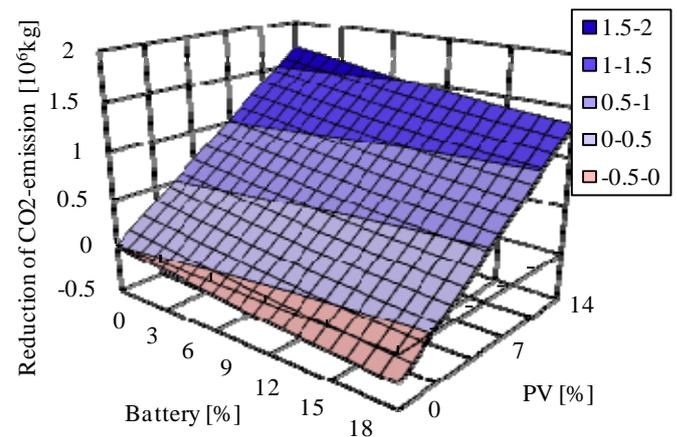
Fig.11 Reduction of total CO2 depending on BESS and PV
