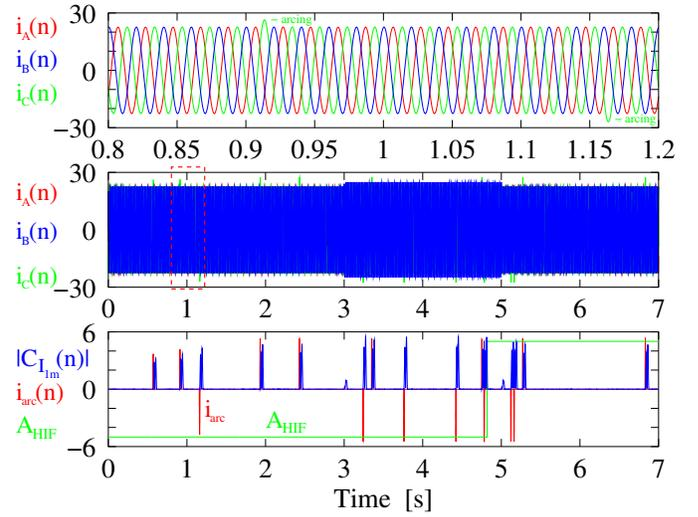
Fig. 6. Sparking high impedance fault detection results, case 2
