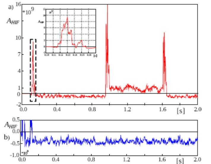
Fig. 4. HIF alarm signals  $A_{HIF}$ , in case of switching heavily loaded feeder 5 and HIF, measured in faulty feeder 5—a) and sound feeder 4—b)
