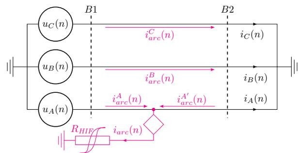
Fig. 1. Arc represented as a current source and a current flow at HIF
