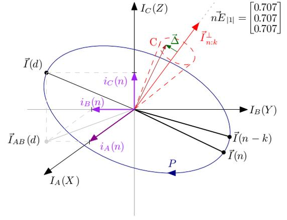
Fig. 3. Graphic presentation of 3D power protection scheme basic vectors and their construction
