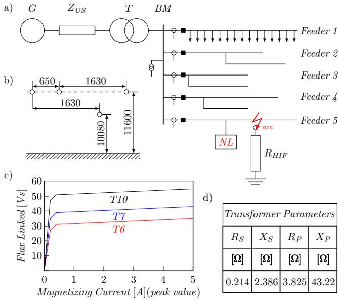
Fig. 7. One line diagram of the test model a), geometrical data for feeder wires configuration (all dimensions in [mm]) b), magnetizing characteristics of a transformer core c) and transformer leakage impedance parameters d)
