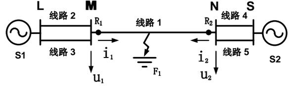
Fig. 4 750kV transmission line system equivalent circuit
