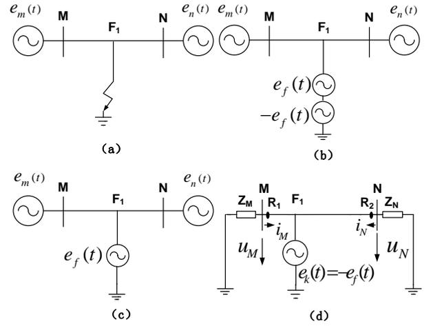
Fig. 2 Superposition theorem Schematic circuit
