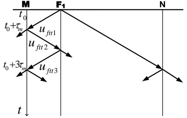
Fig. 3 Lattice diagram of travelling waves for internal fault
