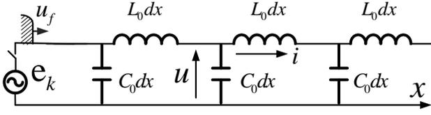
Fig. 1 Distributed parameter equivalent circuit and propagation of fault travelling waves for a single line
