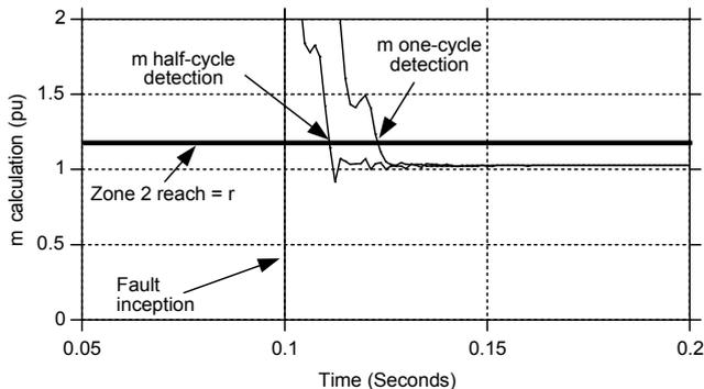
Figure 3.  $m$  Calculations for a Zone 2 A-Phase-to-Ground Fault
