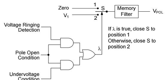
Figure 10. The Relay Inputs Zeros to the Memory Filter When Input Voltages are Corrupted
