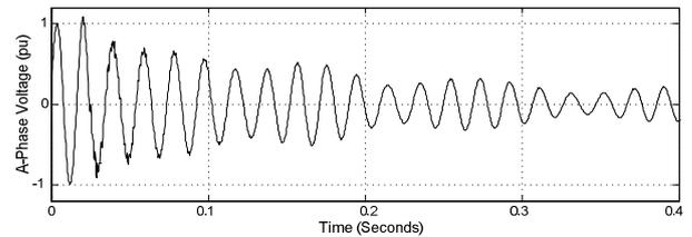
Figure 9. A-Phase Line Voltage After Line De-energization
