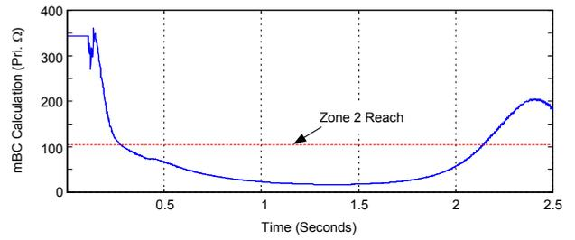
Figure 14. Distance Element Apparent Impedance During Pole-Open Conditions
