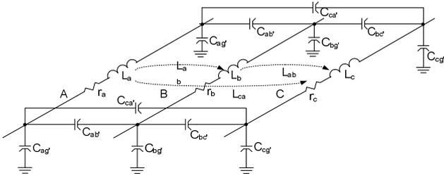
Figure 17. Transmission Line Pi Equivalent Circuit
