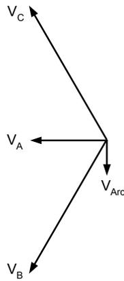
Figure 21. Line Voltages During the Pole-Open Condition
