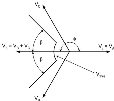
Figure 22. The Angle  $\phi = 180^\circ$  and  $V_\gamma$  is Outside of the SAED Region for Normal Conditions
