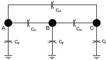
Figure 18. Equivalent Circuit Considering Only the Line Capacitances
