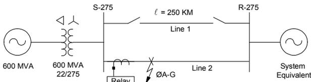
Figure 12. 275 kV Network With 600 MVA Generator
