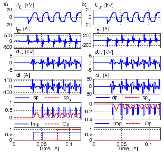
Figure 9. The protection signals in a damaged TL4 line (a) and a "healthy" K1 line (b) during a short circuit with two arc ignition per cycle at the point P4 in a network with isolated neutral point (arc ignition voltage  $U_{ig} = 8$  kV)
