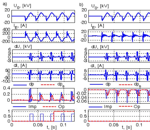
Figure 8. The protection signals in a damaged K2 line (a) and a "healthy" TL3 line (b) during a short circuit at the point PK21 in a network whose neutral point is grounded with a resistor  $R_N = 58$  Ohm (150 A)
