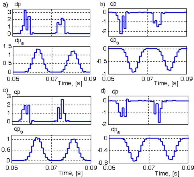
Figure 10. Power impulses of details in a damaged K2 line (a) and a "healthy" K1 line (b) without angular error and with error 4,5 degrees (c, d) during short circuit at the point PK21 in a network with isolated neutral point (arc ignition voltage  $U_{ig} = 20$  kV)
