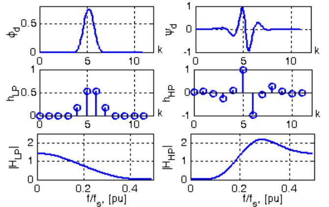
Figure 3. Wavelet of rbio3.5 type  $\psi_0$ , its scaling function  $\phi_0$ , impulse responses and amplitude spectra of filters LP and HP for decompositions associated with this wavelet
