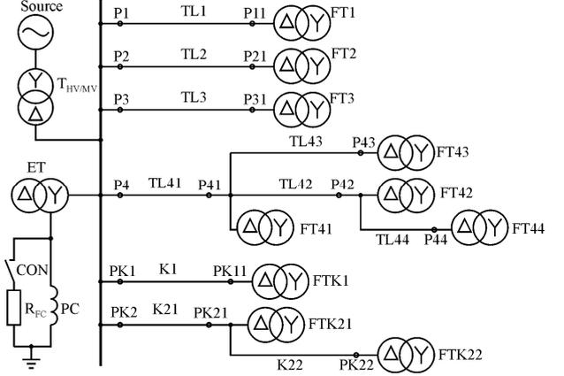
Figure 2. General diagram of the modelled MV network
