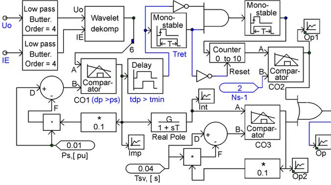
Figure 5. A simplified model of protection using the wavelet criteria
