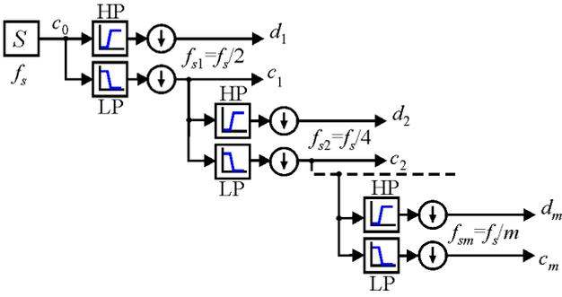
Figure 1. Diagram of multi-resolution wavelet decomposition
