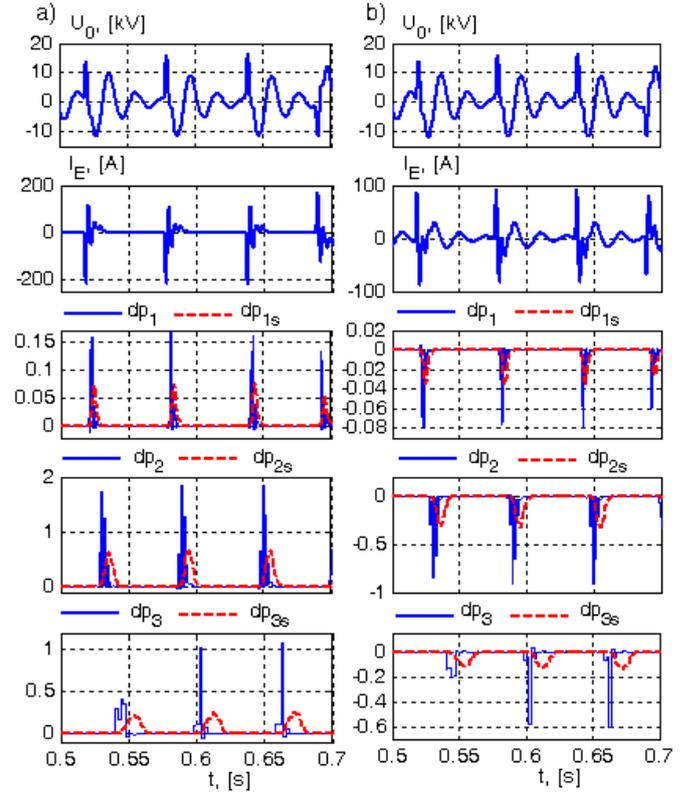
Figure 4. Zero sequence voltage and currents and signals of instantaneous power of details at three levels of decomposition: a) on the line TL4 with earth short circuit; b) on the “healthy” line K2
