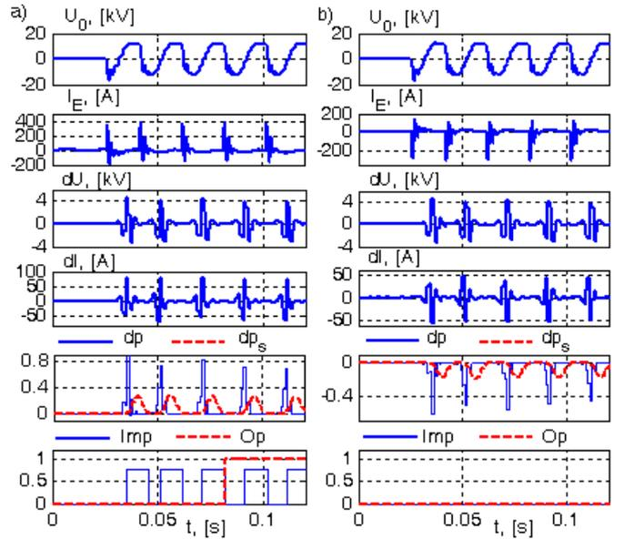
Figure 6. The protection signals in a damaged K2 line (a) and a “healthy” K1 line (b) during a short circuit at the point PK2 in a network with isolated neutral point
