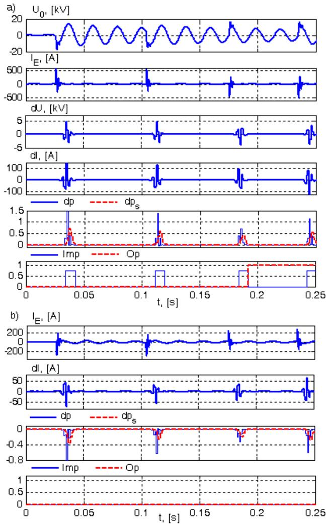
Figure 7. The protection signals in a damaged TL4 line (a) and a "healthy" K2 line (b) during a short circuit at the point P41 in a compensated network ( $s = -0,1$ )
