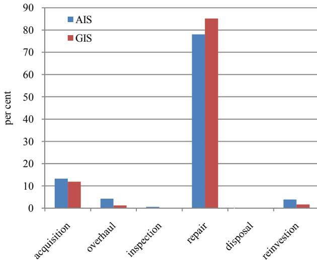
Figure 4: Present value of circuit breakers for AIS and GIS
