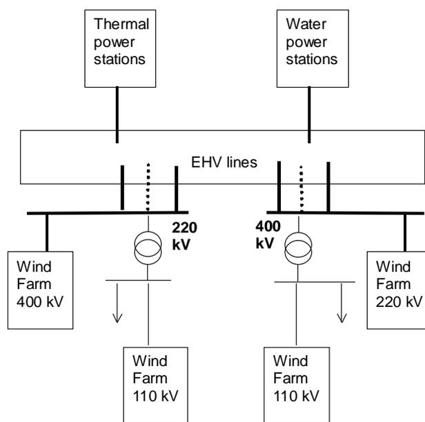
Figure 1. The interconnection of wind farms to the transmission network
