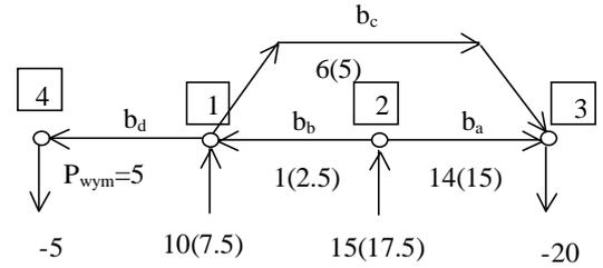
Figure 2. Power flow resulting from optimal wind farms power selection. In brackets the farm powers and power flow fulfilling the system constraints have been given.
