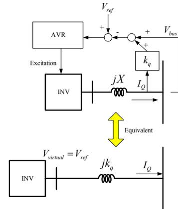
Fig. 2 Reactive power control by voltage-source inverter
