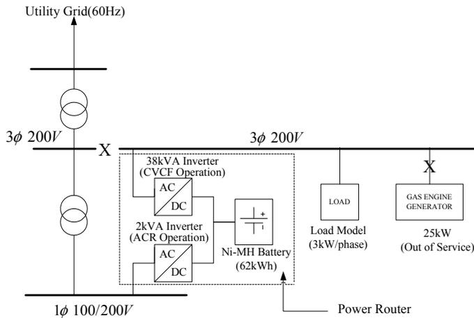
Fig. 8 Laboratory test diagram
