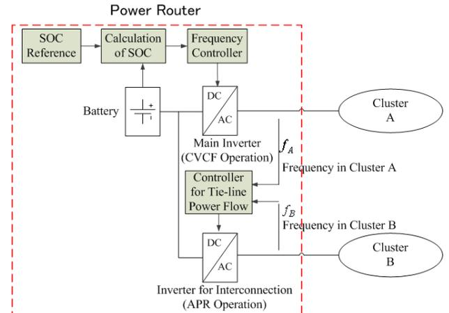
Fig.5 Power Router for control of cluster frequency and tie-line power flow
