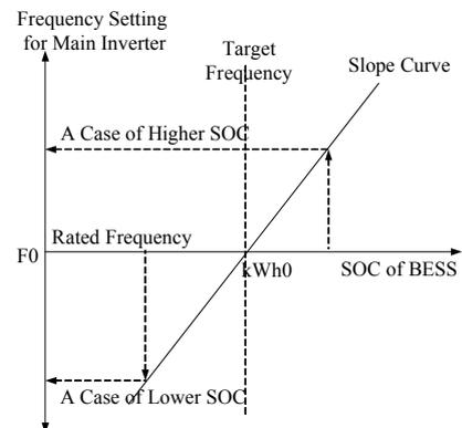
Fig.6 An example of frequency setting for main inverter with SOC
