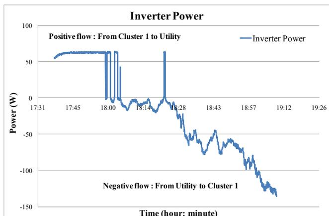
(b) Power flow in 2kVA inverter
