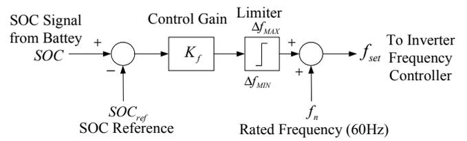
(a) Frequency control in 38kVA inverter (CVCF operation)
