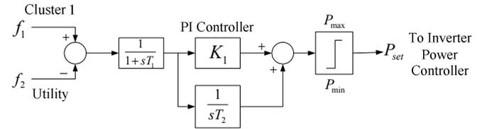
$K_1 = 0.25(kW / Hz)$ ,  $T_1 = 30(s)$ ,  $T_2 = 99999(s)$ ,  $P_{max} = 1(kW)$ ,  $P_{min} = -1(kW)$
