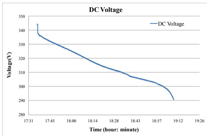
(c) DC side voltage in the Power Router
