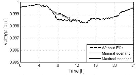
Figure 8. Voltage profile at node u (at power supply)
