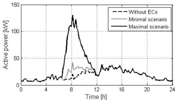
Figure 4. Load profiles for active power at node b6 (at parking lot)
