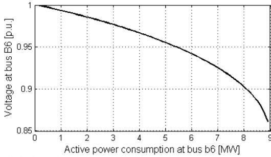
Figure 6. Voltage instability at 10kV bus B6 due to rising power consumption ( $\cos\phi=0.68$ ) at bus b6
