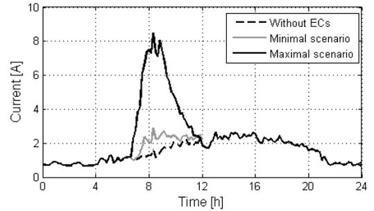
Figure 9. Currents in Line 5 for different scenarios
