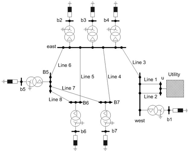
Figure 1. Topology of the modeled distribution power system
