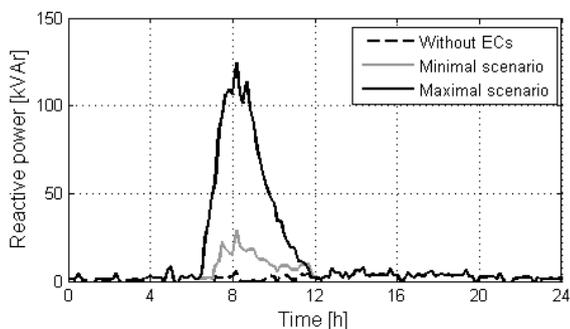
Figure 5. Load profiles for reactive power at node b6 (at parking lot)
