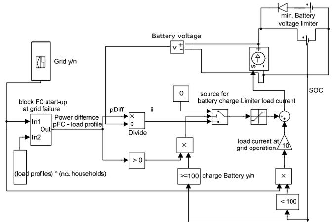
Figure 4. Dynamic Matlab model of the decentralized power system comprising fuel cell and battery
