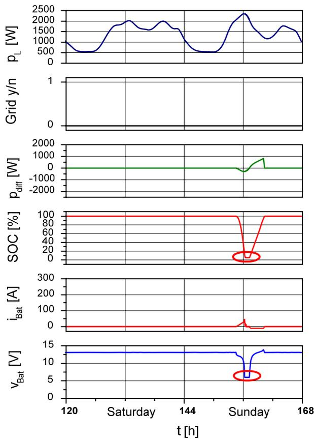
Figure 10. Island operation with standardized load profile for 11 households (summer) – operation is interrupted
