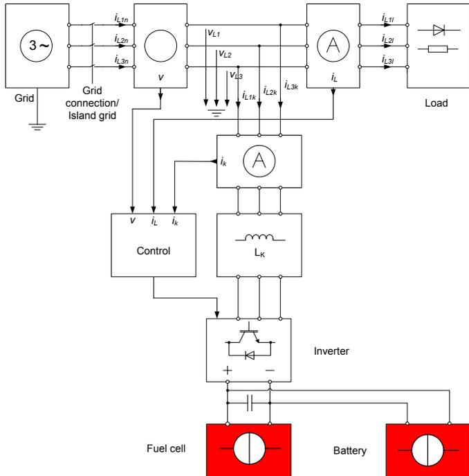
Figure 3. Decentralized power system (model)
