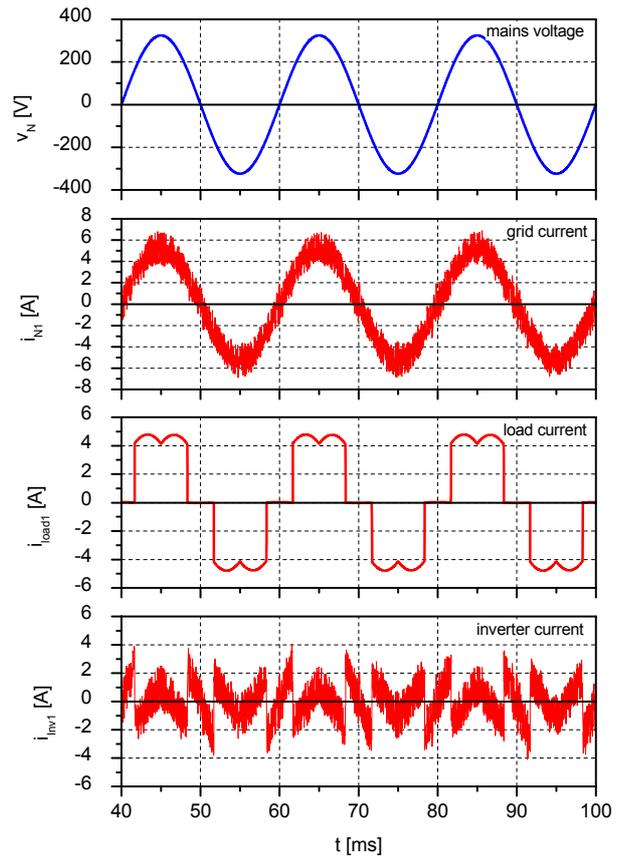
Figure 11. Simulation of power factor correction for a B6U rectification with resistive load, only one phase is shown
