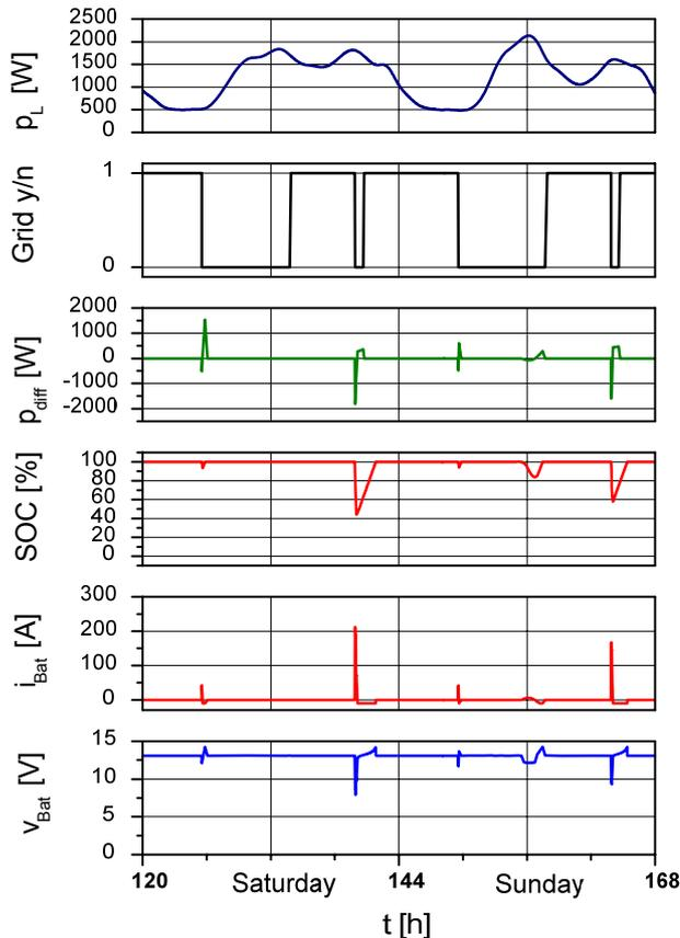
Figure 8. Grid failures with standardized load profile for 10 households (summer) – uninterrupted subnetwork operation is maintained
