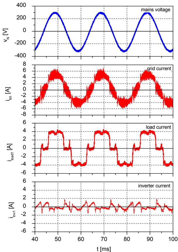
Figure 12. Measurement of power factor correction for a B6U rectification with resistive load, only one phase is shown
