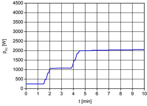
Figure 2. Start-up of a 5.2 kW LT PEM fuel cell to a thermal stable operating point at 2.06 kW
