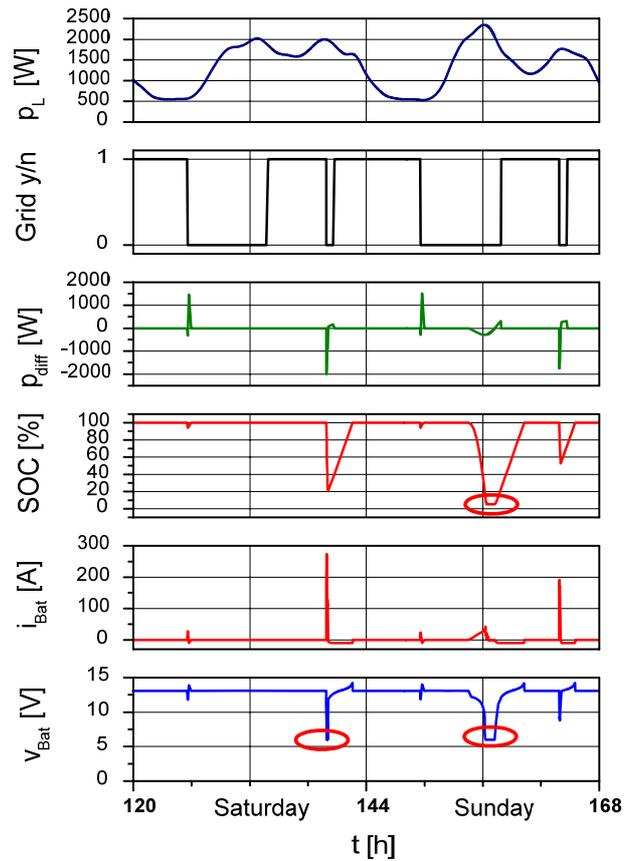
Figure 9. Grid failures with standardized load profile for 11 households (summer) – subnetwork operation is interrupted
