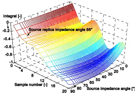
Figure 7. Sensitivity of the direction method for a different replica impedance angle
