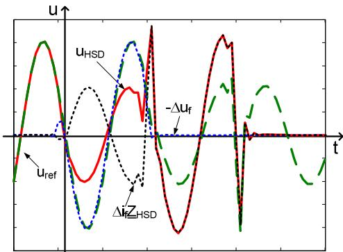
Figure 16. Evolving fault during the same phase AN reverse to AN forward
