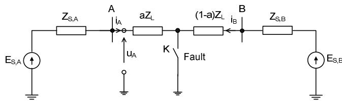
Figure 1. Schematic representation of electrical circuit structure change after fault on the line
