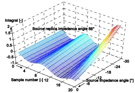
Figure 8. Sensitivity of the direction method for a different replica impedance angle
