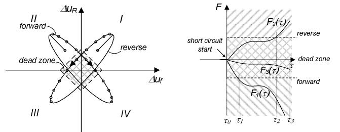
Figure 6. Trajectories and curves of the directional element based on delta-quantities
