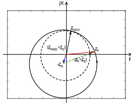
Figure 9. Distance characteristic for the forward fault (HSD-method)
