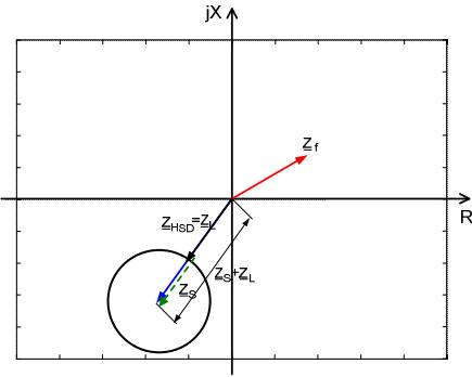
Figure 10. Distance characteristic for the reverse fault (HSD-method)
