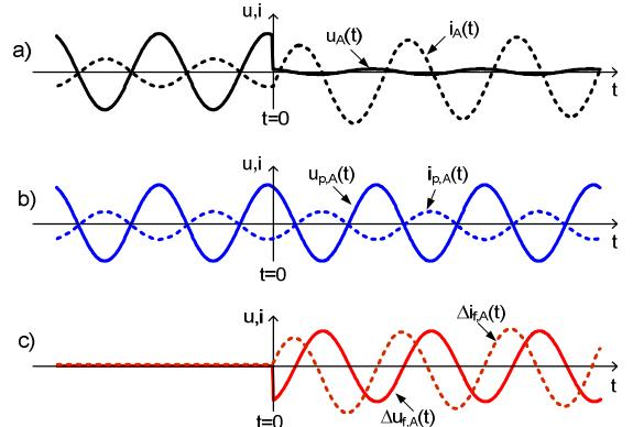
Figure 4. Electrical quantities during fault event: a) voltage and current before and after short circuit; b) voltage and current without short circuit; c) delta-voltage and delta-current.
