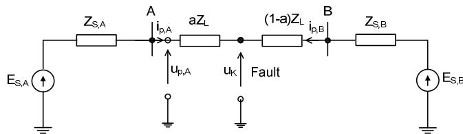
Figure 2. Schematic representation of an electrical circuit in the form of the pre-fault quantities
