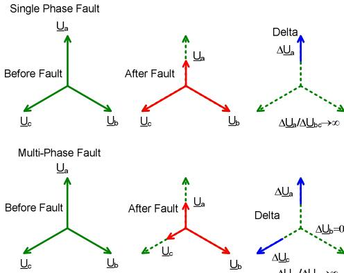
Figure 5. Loop selection based on the delta-voltage
