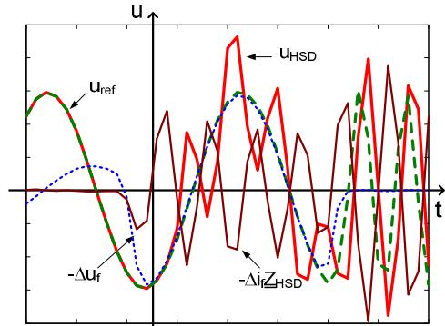
Figure 14. Reverse fault with significant disturbance content
