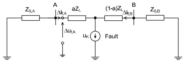
Figure 3. Schematic representation of the electrical circuit in the form of the delta-quantities
