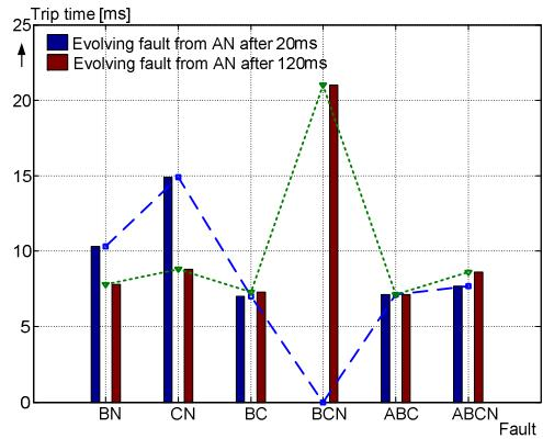
Figure 15. Results of the evolving fault tests
