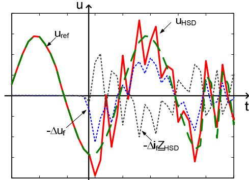
Figure 13. External Fault at >100% line length with significant disturbances content
