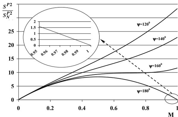
Fig.2 The relative serial converter power load during short circuit as a function of its intrusion voltage (relative absolute value  $M$  and phase  $\Psi$ )
