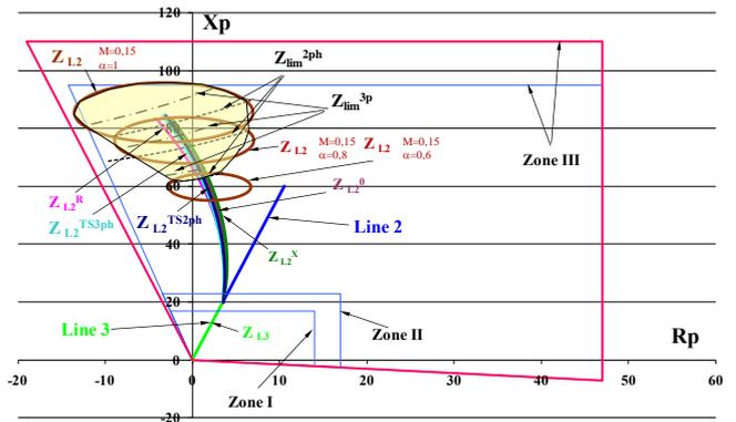
Fig.6 The measured impedance by protection AP6 at metallic short-circuit in line L2 for negative angle  $\delta_{31}$
