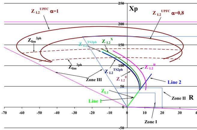
Fig.4 The measured impedance by protection AP1 at metallic short-circuit in line L2 for negative angle  $\delta_{13}$
