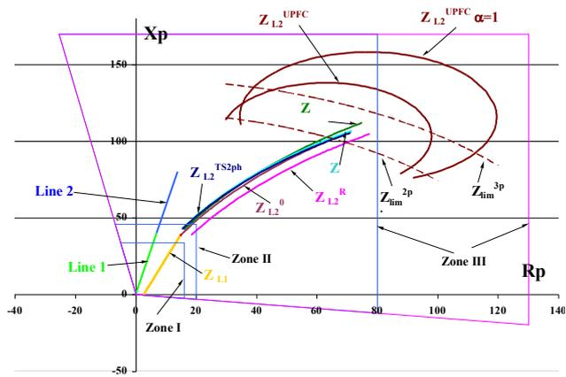
Fig.5 The measured impedance by protection AP1 at arc short-circuit in line L2 for positive angle  $\delta_{13}$
