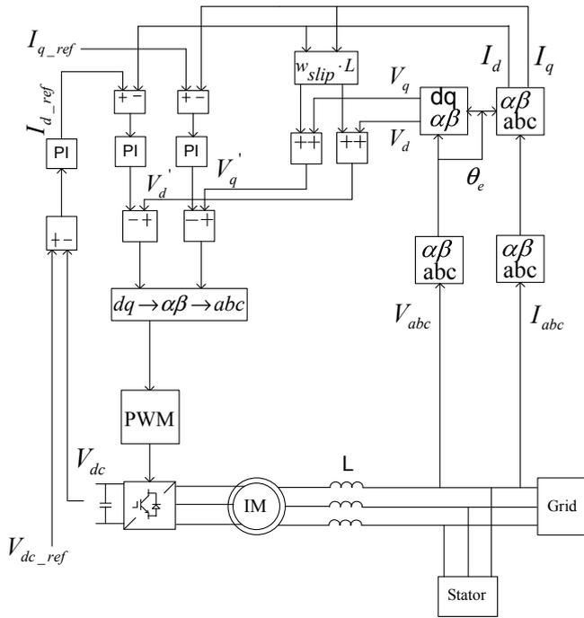
Figure 3. Structure of control system for grid side converter
