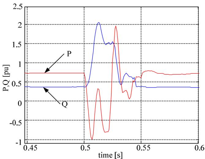
Figure 14. Active and reactive power in the grid
