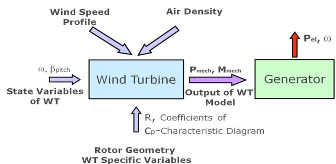
Figure. 1. General structure of the wind turbine model
