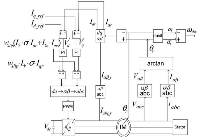
Figure 4. Structure of control system for rotor side converter
