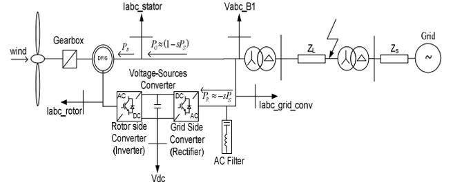
Figure 2. Detailed structure of the considered WT model
