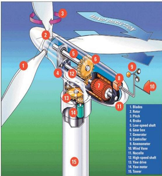
Fig. 11. Various components of a wind power system [17].
