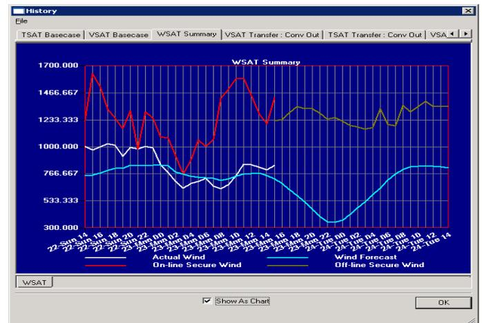
Fig. 4. WSAT summary: Red curve is a RT secure wind limit based on the lowest security limit; Golden curve is FC wind limit for next 24 hours; White curve is actual wind generation; and Blue curve is wind generation forecast. All data is in MW.
