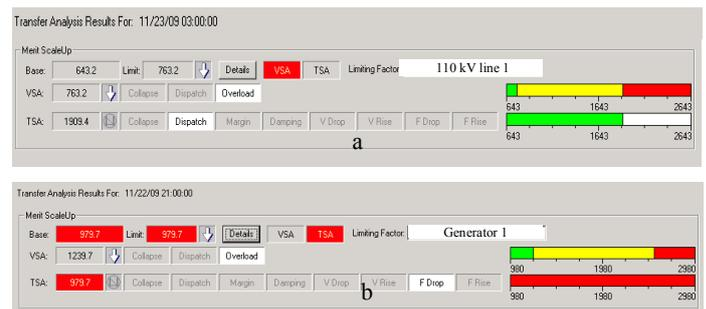
Fig. 5 Visualizations of transfer limits; green area – safe transfer; yellow area – the security criteria is violated; red – collapse: a) Overload due to “110 kV line 1” N-1 contingency in VSA Merit ScaleUp transfer; b) Frequency criterion (F Drop) violation due to Unit 1 trip in TSA Merit ScaleUp transfer
