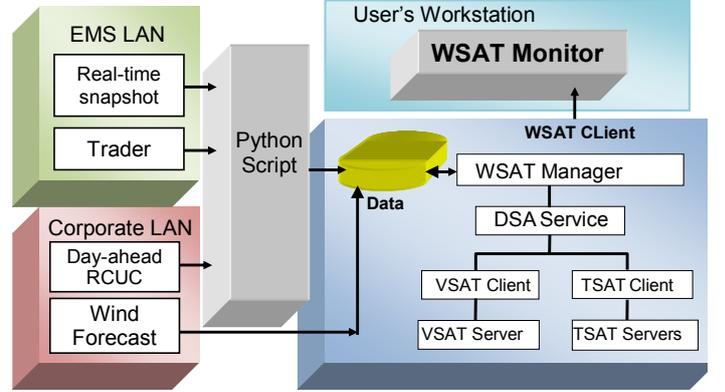
Fig. 2. WSAT software structure
