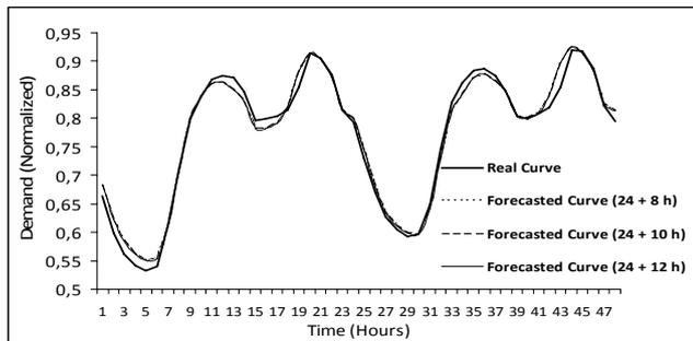
Figure 9. Forecasted curves with different testing input data patterns (24+8h, 24+10h, and 24+12 h) vs. Real curve of the 7<sup>th</sup> week of 2004.
