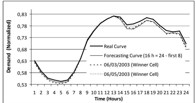
Figure 5. Real load demand (06/16/04) vs Estimated load curve (Average of the winner cell corresponding to labels 06/03/03 and 06/05/03).
