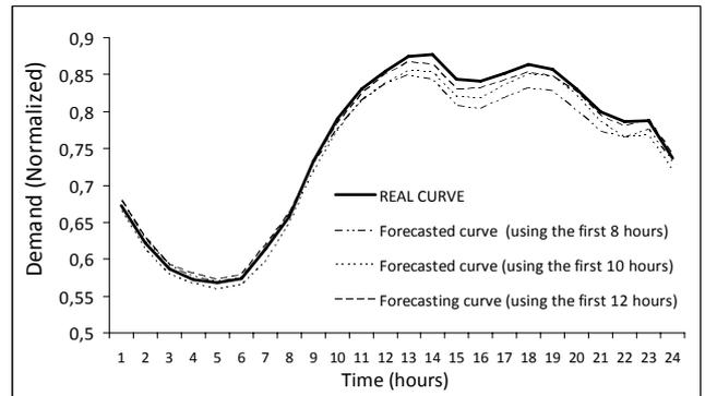
Figure 6. Real load demand curve vs Estimated load curve using 8, 10 and 12 hours as input data (07/15/04).
