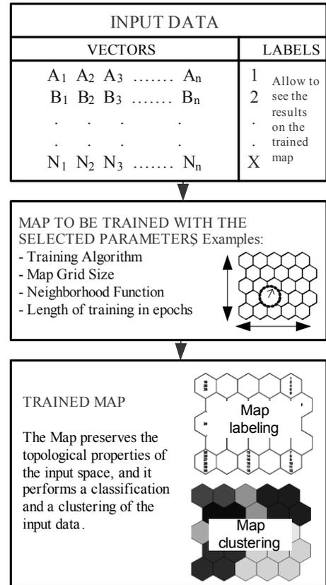
Figure 2. Steps for application of the SOM.
