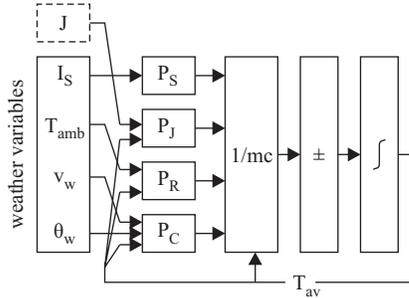
Fig. 10. Overview of the dynamic thermal model
