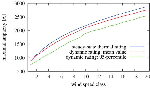
Fig. 14. Comparison of the steady-state and dynamic approach in weather-based loading
