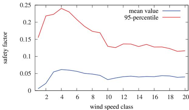
Fig. 15. Applicable safety factors for correction of the steady-state thermal rating
