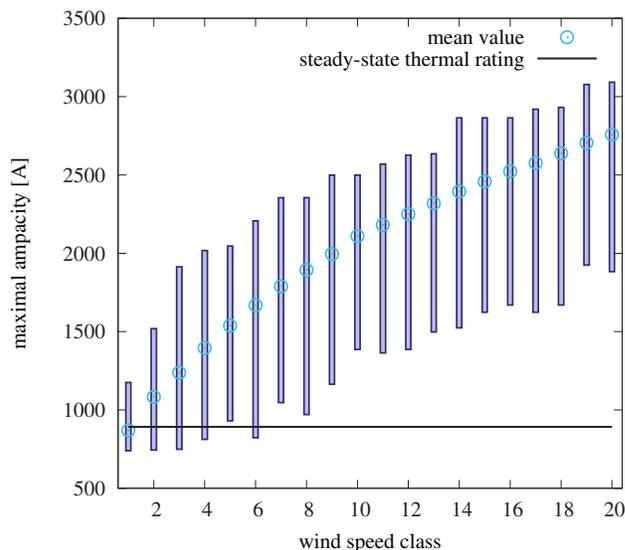
Fig. 12. Maximal ampacity for the different wind speed classes
