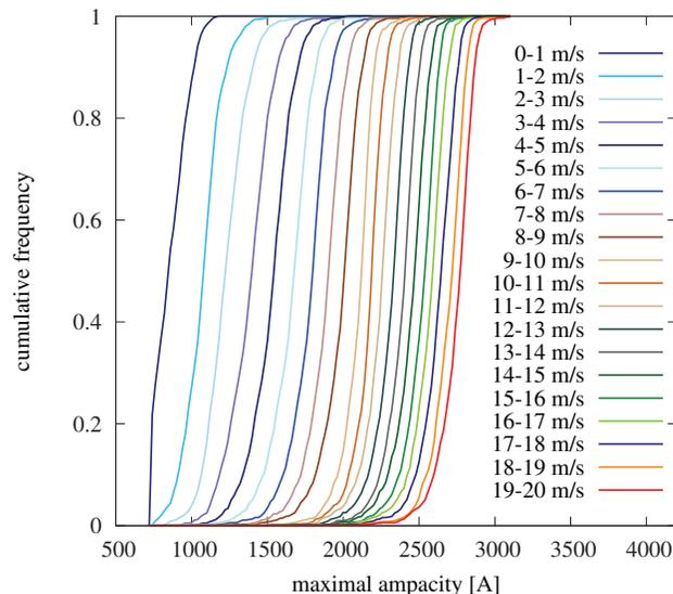
Fig. 13. Probability functions of the calculated ampacity for the different wind speed classes
