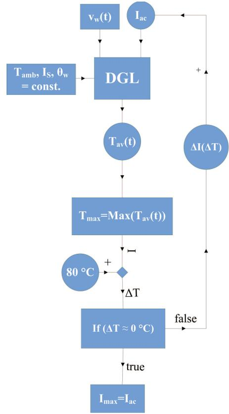
Fig. 11. Flowchart of the algorithm as applied to the case study of section IV
