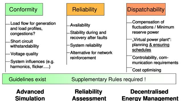
Figure 2. Requirements means for a large scale penetration of DER [12].
