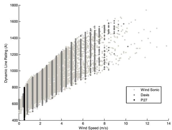
Fig. 5 Scatter plot to show the difference in calculated dynamic line rating using wind speeds from P27 standard (0.5m/s) compared with the Davis anemometer and the Windsonic
