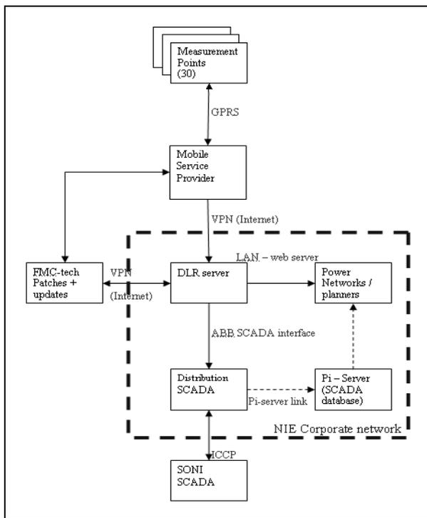
Fig. 9 System architecture for control centre integration of DLR
