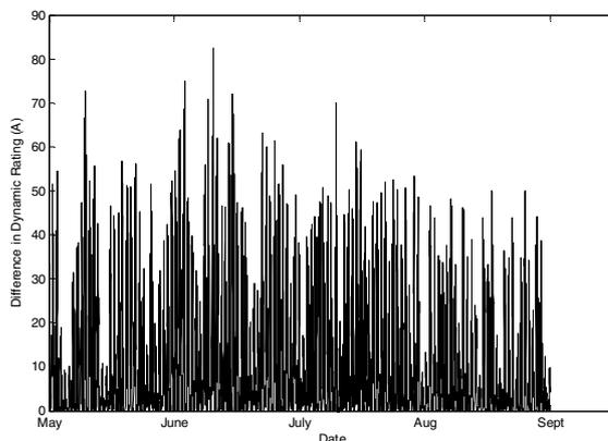
Fig. 8 Difference in using P27 zero solar factoring and NIE's method of calculating solar heating in calculating the Dynamic Line Rating
