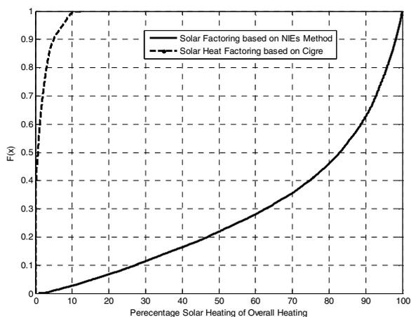
Fig. 6 Difference in using Cigré and NIE's method for factoring solar heating
