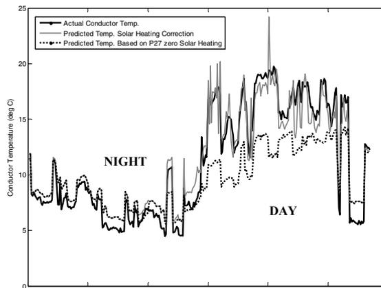
Fig.7 Difference in predicting the conductor temperature using zero solar radiation compared with the more accurate method NIE use
