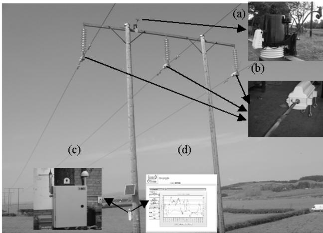
Fig. 4 Photograph of (a) weather station, (b) line mounted sensors, (c) X-NET controller and (d) web controller screen shot
