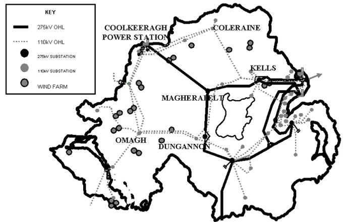
Fig. 3 Map of Northern Ireland transmission grid with wind farm locations up to the end of 2009 superimposed
